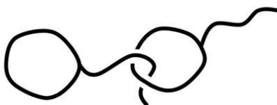
Figure 4-3. Schematic illustration of the intermolecular ring-linear penetration of single-tail tadpole molecules. Reprinted with permission from ref. 1.
