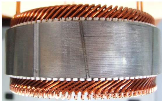
Fig. 6.1 Rectangular wire motor stator without varnish treatment
