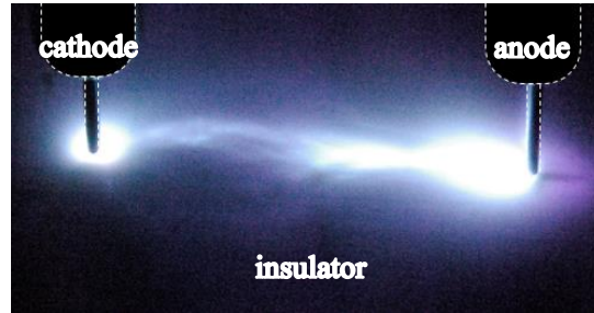
(a) Still image of surface flashover of c-i-a
