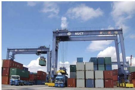
(2) Yard Cranes: A transfer crane (left) and a straddle carrier (right)
