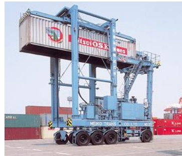
(2) Yard Cranes: A transfer crane (left) and a straddle carrier (right)
