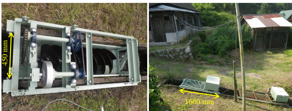
Fig. 1.3. The image of the Archimedes screw hydropower system in the open and inclined channel.
