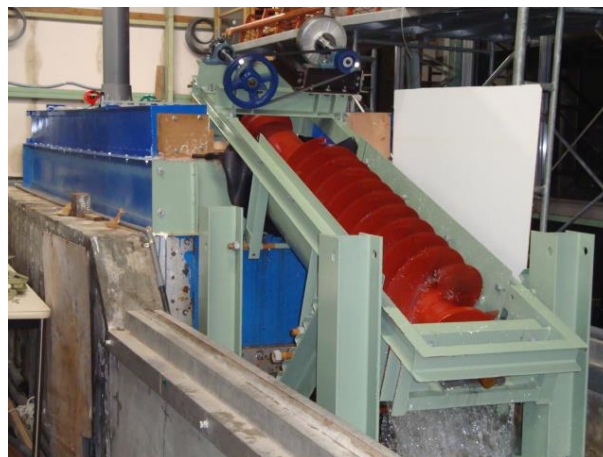
Fig. 3.8. The experimental equipment of the Archimedes screw hydropower system in the variable inclined open channel.
