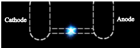
Figure 4. Still image of breakdown for c-a ( V_{BD} = -20.8 \text{ kV} , g=0.25 \text{ mm} , d=28.5 \text{ mm} )
