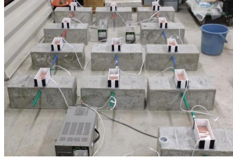
Fig. 4. Electric corrosion test using NaCl ponds
