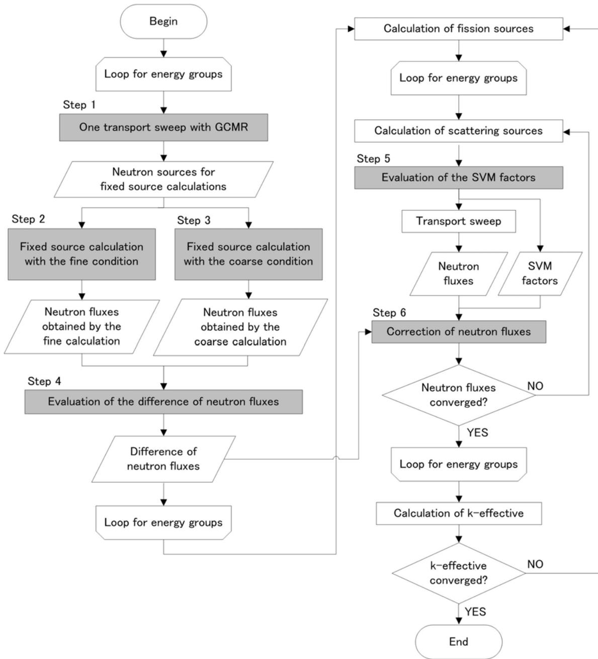
Figure 2. Flow chart for the calculation procedure of the SVM method.
