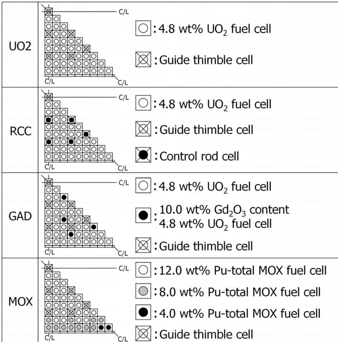
Figure 3. Geometries for single assembly calculations.
