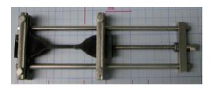
Fig. 2: Dumbbell specimen with pre-strain
