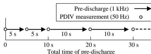
Figure 3. PDIV measurement procedure.
