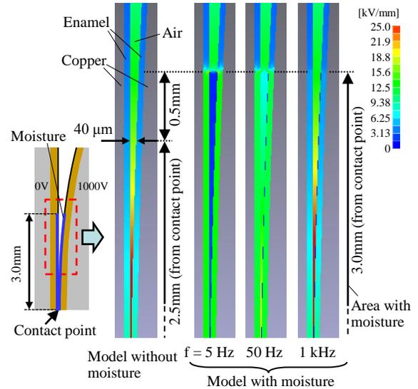
Figure 14. Electric field distribution for different frequencies (Moisture layer is attached to coil coating containing contact point).
