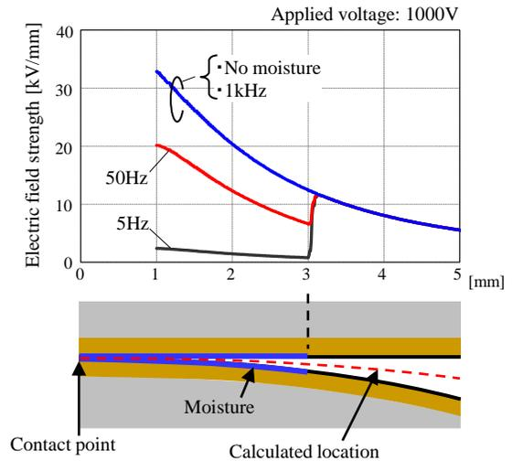
Figure 15. Electric field strength when moisture layer is attached to coil coating containing contact point.
