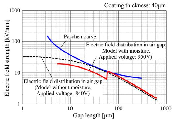
Figure 16. Relationship between electric field distribution in air gap and Paschen curve (Moisture layer is attached to coil coating containing contact point).
