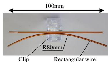
Figure 2. Test sample.
