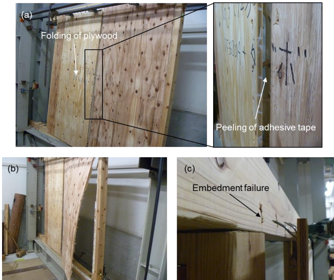
Figure 6.8 Failure mode of shear wall specimens. (a), (b)W-T1D and W-T2D, (c) W-N.
