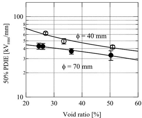
Fig. 4 Void ratio dependence of 50% PDIE of Tyvek<sup>®</sup> in LN<sub>2</sub> for different electrode diameters
