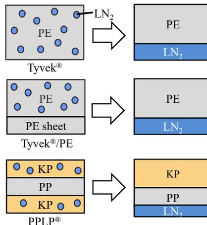
Fig. 3 Calculation models of test samples immersed in LN<sub>2</sub> for electric field analysis
