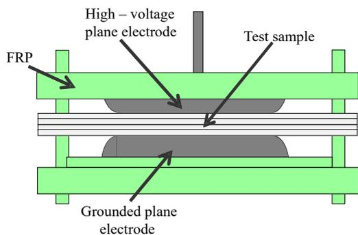
Fig. 2 Test sample configuration
