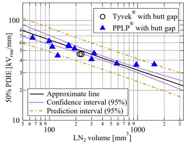
Fig. 8 50% PDIE as a function of LN<sub>2</sub> volume for different porous papers with butt gaps in LN<sub>2</sub>
