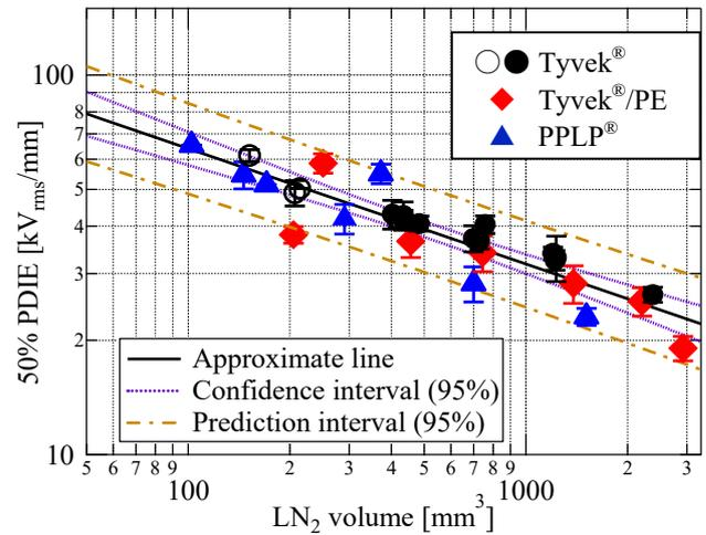
Fig. 6 50% PDIE as a function of LN<sub>2</sub> volume for different porous papers in LN<sub>2</sub>
