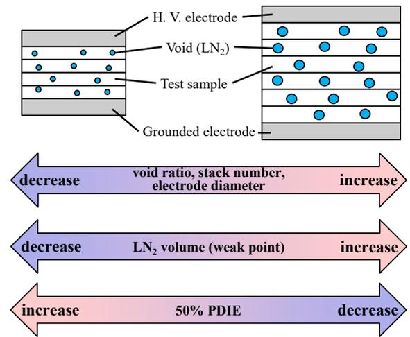
Fig. 7 Schematic illustration of volume effect in porous papers immersed in LN<sub>2</sub>
