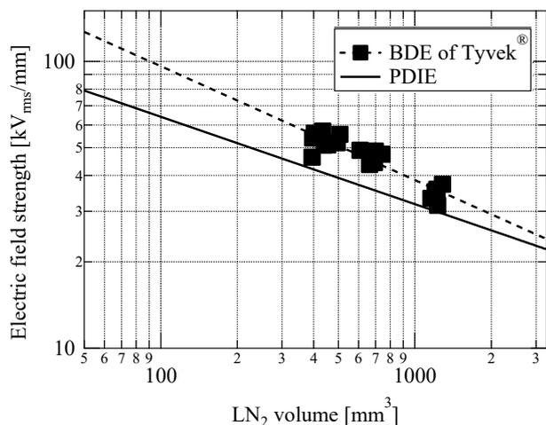
Fig. 8 Comparison of 50% PDIE and BDE of Tyvek® in LN<sub>2</sub>
