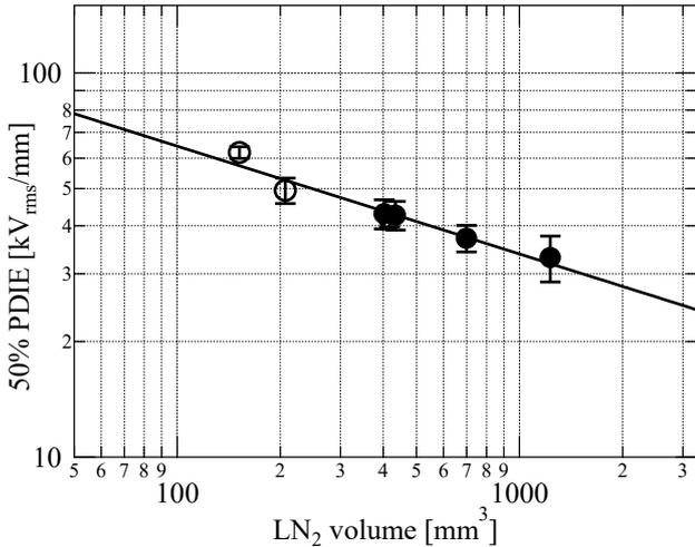
Fig. 5 50% PDIE as function of LN<sub>2</sub> volume in Tyvek<sup>®</sup> immersed in LN<sub>2</sub>
