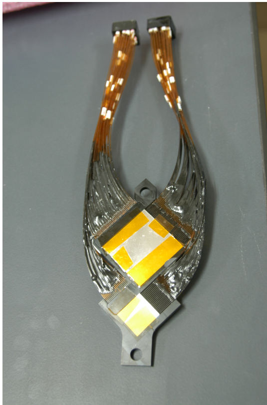
Figure 2.6: A completed one layer of the GSO-bar hodoscope. Fibers from the GSO-bars are bundled with epoxy glue.
