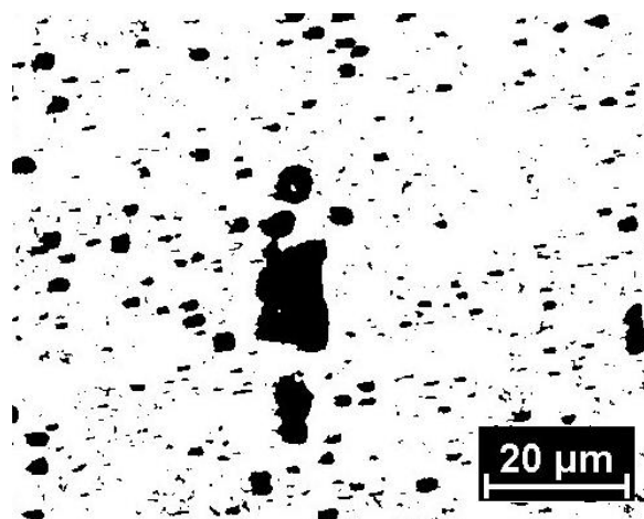
Fig. 5.3 Binary image of metallographic photograph of DC53.
