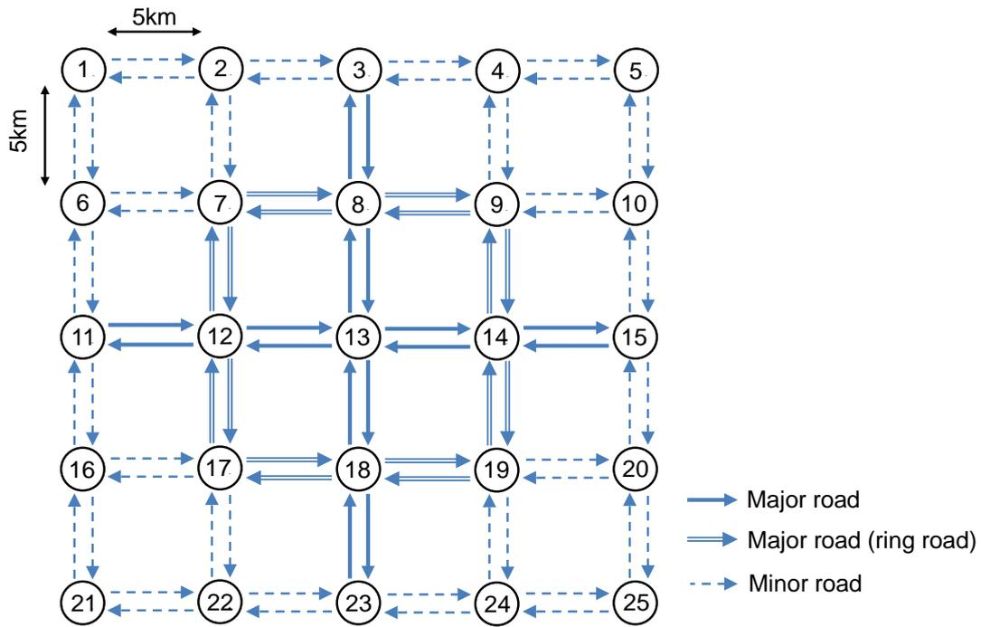
**Fig. 3.** Grid network for test simulation
