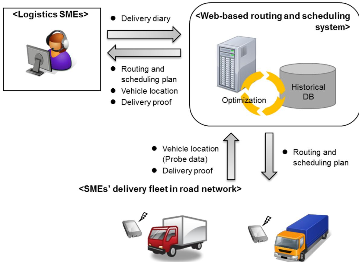
**Fig. 1.** Components of web-based dynamic routing and scheduling system for SMEs
