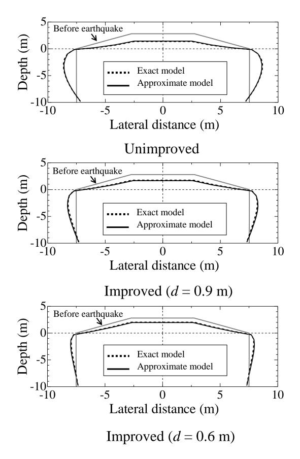
Fig. 14. Deformations of improved region and embankment.
