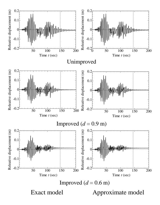
Fig. 12. Relative displacement responses (x direction).
