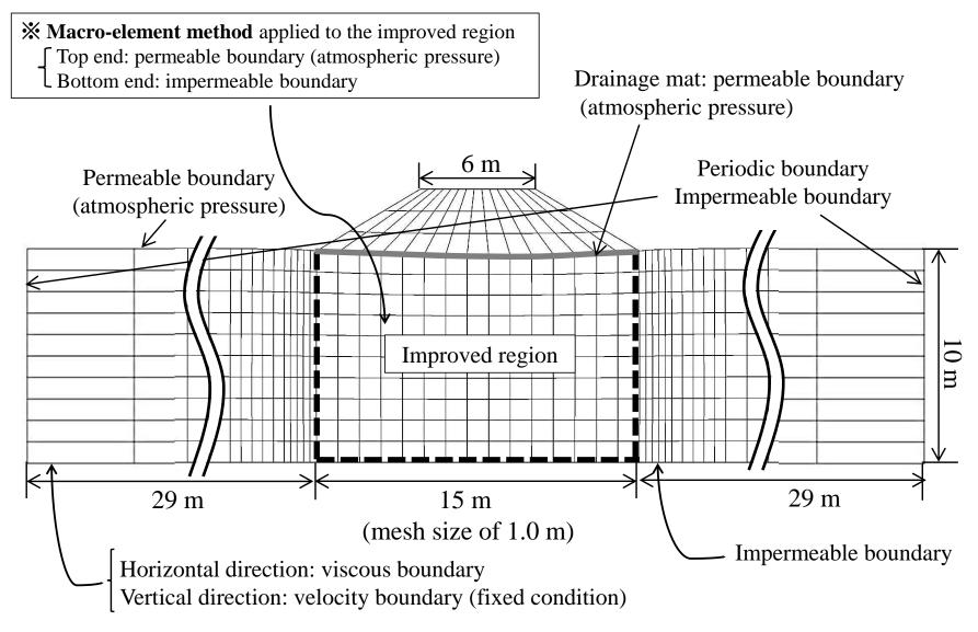
Fig. 4. Finite element mesh and boundary conditions (approximate model).
