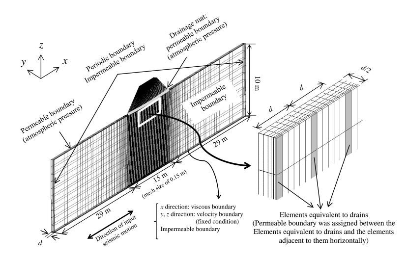
Fig. 3. Finite element mesh and boundary conditions (exact model).
