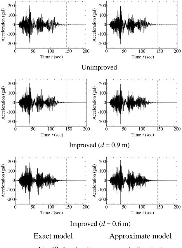
Fig. 10. Acceleration responses (x direction).
