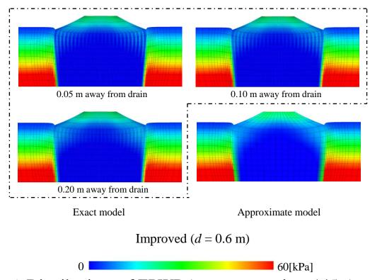
Fig. 6. Distributions of EPWP (x-z cross section, 145 s).
