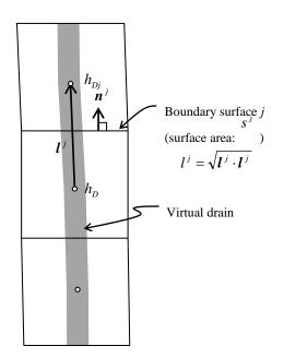
Fig. 1. Virtual drain contained in mesh.
