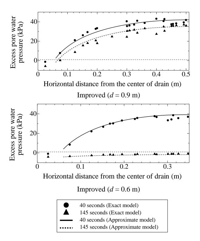
Fig. 9. EPWP along the distance from the center of drain.
