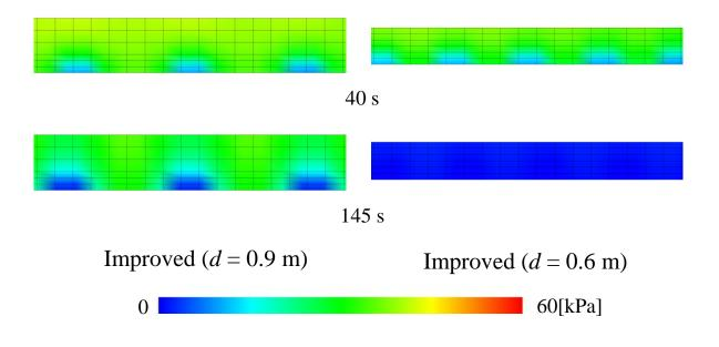
Fig. 8. Distributions of EPWP (x-y cross section, Depth 4.5 m).
