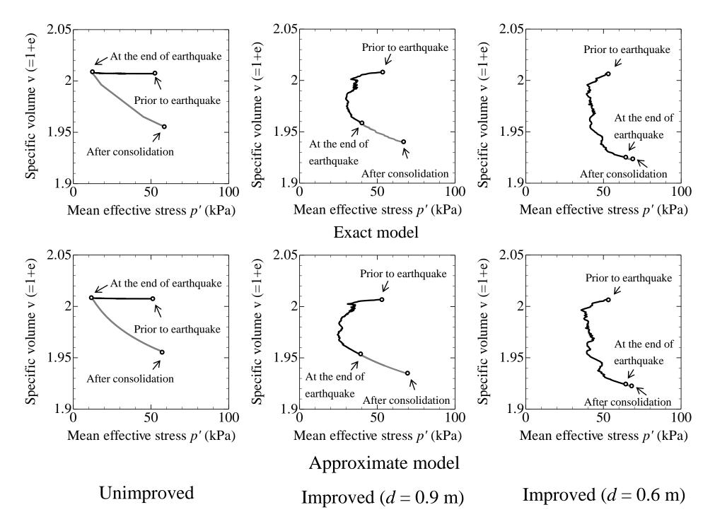
Fig. 15. Relationships between the mean effective stress and the specific volume.
