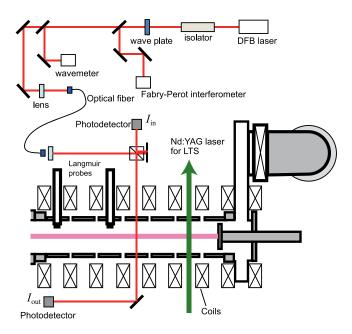
FIG. 2. A schematic of the LAS system in NAGDIS-II.
