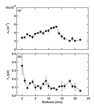
FIG. 4. Radial profiles of (a) the electron density and (b) temperature measured by the LTS.
