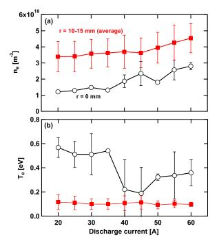
FIG. 5. Discharge current dependences of (a) the electron density and (b) temperature at r = 0 and 10-15 mm (averaged values).
