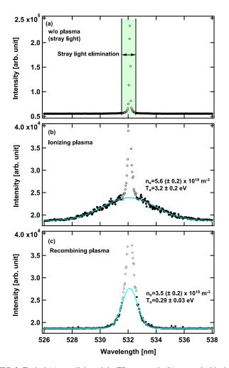
FIG. 3. Typical (a) stray light and the TS spectrum in (b) an attached ionizing plasma and (c) a detached recombining plasma, respectively.
