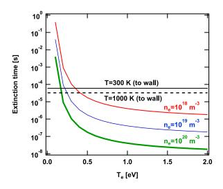
FIG. 7. The characteristic time of neutral transport in NAGDIS-II and the extinction time of the  $2^{3}S$  state atoms as a function of the electron temperature.
