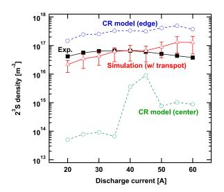
FIG. 9. Comparisons of experimentally obtained and calculated 2<sup>3</sup>S densities as a function of the discharge current.
