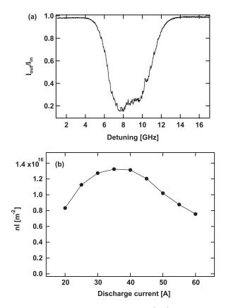
FIG. 6. (a) A typical absorption spectrum for  $2^{3}S-3^{3}P$  transition in the detached plasma in NAGDIS-II and (b) the discharge current dependence of the line integrated  $2^{3}S$  density when the laser was aligned at the center.
