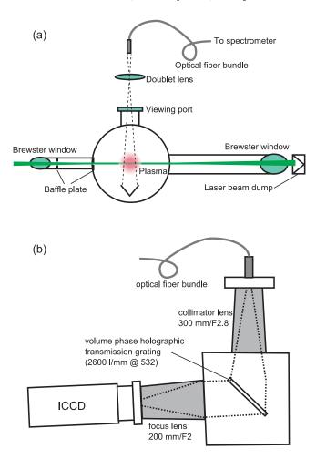
FIG. 1. (a) A schematic of the laser path and the collection optics for the LTS in the NAGDIS-II device, and (b) a schematic of the spectrometer for the LTS.
