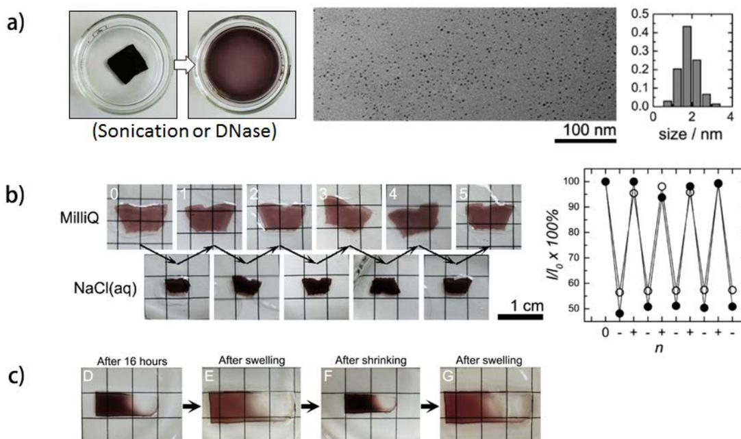
**Figure 5.** (a) Photographic images of metallized DNA hydrogel before after dispersion into aqueous solution, TEM images of gold nanoparticles obtained by DNA hydrogel dispersion and typical distribution of their sizes (Adapted with permission from Che, Y.; Zinchenko, A.; Murata,
