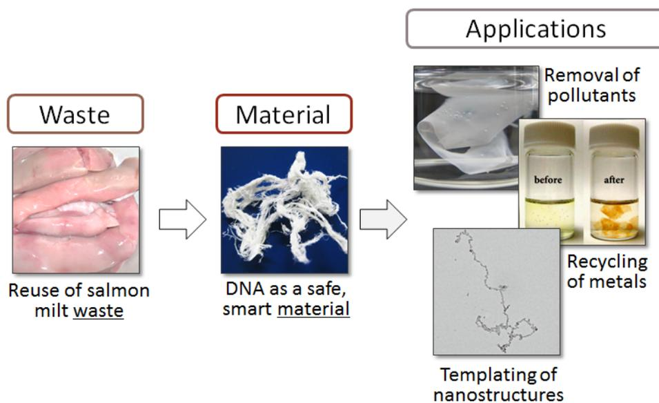
**Figure 1.** Application of DNA as a material. Extraction of DNA from waste salmon milt is used to obtain large quantities of DNA that are further used for materials science and environmental applications.
