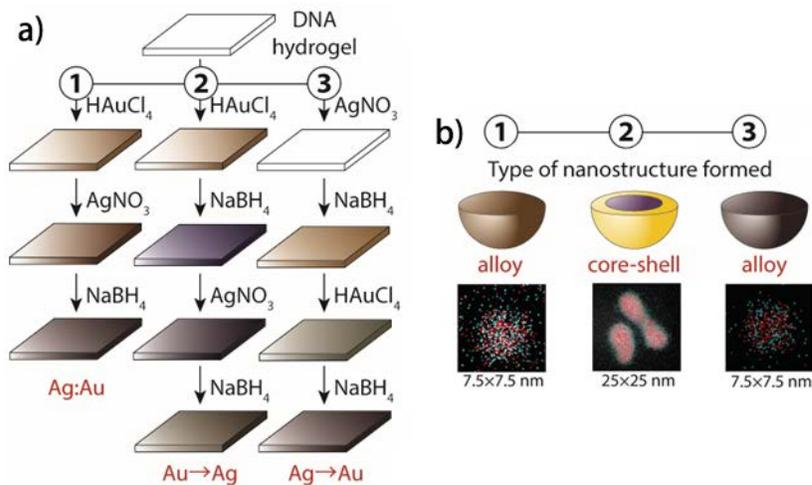
**Figure 6.** (a) Schematic outline of three routes to prepare Ag-Au bimetallic nanostructures inside DNA hydrogels<sup>69</sup>. (b) Type of bimetallic NP formed inside DNA hydrogels according to three routes shown in (a) and corresponding element mapping (HAADF-STEM) of Ag (red) and Au (blue) elements in the obtained NPs. (Adapted with permission from Taniguchi, S.; Zinchenko, A.; Murata, S., Chem. Lett. 2016, 45 (6), 610-612, Copyright the Chemical Society of Japan)
