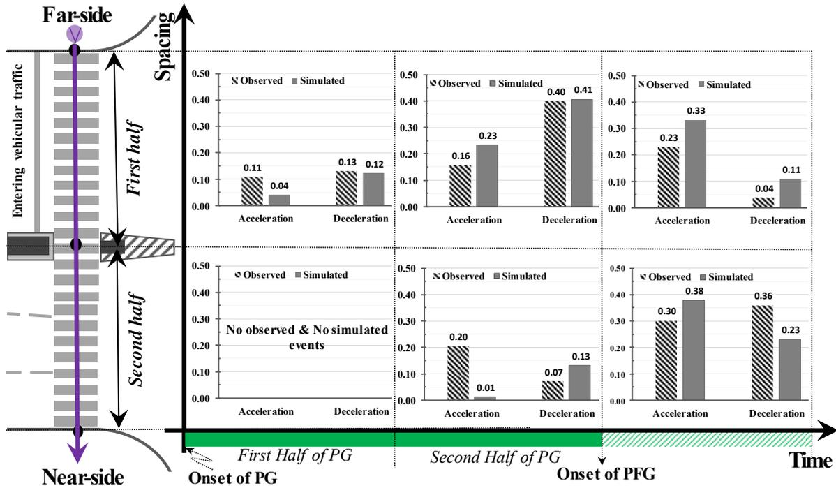
Figure 10. Comparison between observed and simulated probabilities of speed change events considering timing and location at the North crosswalk of Kanayama intersection
