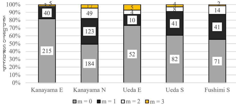
Figure 3. Number of observed speed profiles classified by number of identified speed change events (Iryo-Asano et al. 2015)
