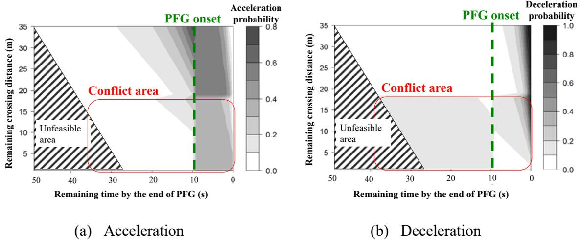
Figure 5. Example of acceleration / deceleration probability contours
