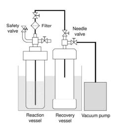
Scheme of laboratory-scale apparatus for dimethyl ether separation.
