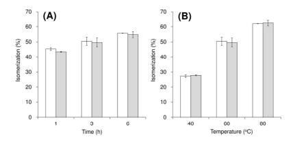
Changes in the total amount of lycopene Z-isomers contents when thermally isomerized at (A) 60 °C for 1, 3, and 6 h, and (B) 40, 60, and 80 °C for 3 h in hexane (open bars) and dimethyl ether (shaded bars). Isomerization (%) is expressed as a percentage of the amount of Z-isomers in the total amount of lycopene isomers, including (all-E)-lycopene.
