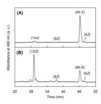
Normal-phase HPLC chromatograms of lycopene isomers after the separation treatment at 4 °C and 0.3 MPa by dimethyl ether, as shown in Figure 2: (A) trapped lycopene in 0.5-µm stainless steel filter, and (B) recovered lycopene in recovery vessel. Before the separation, (all-E)-lycopene was isomerized to the Z-isomers in dimethyl ether at 60 °C for 3 h.
