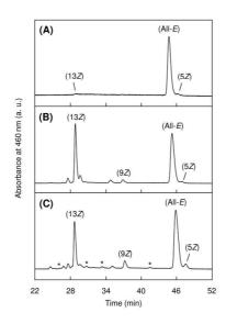
Normal-phase HPLC chromatograms of (A) (all-E)-lycopene and thermally treated lycopene at 60 °C for 3 h in (B) hexane and (C) dimethyl ether. (5Z)-, (9Z)-, and (13Z)-lycopene designated in the charts were identified according to the previous studies. [29-33] Asterisk symbols show the Z-isomer of lycopene peaks which were observed only in DME.
