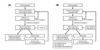
Schematic diagram for procedure comparison of (A) general organic solvent method with (B) DME method to obtain lycopene composition rich in Z-isomers of lycopene.
