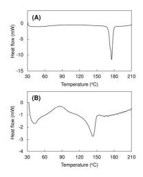
DSC curves of lycopene (A) before and (B) after Z-isomerization in dimethyl ether at 60  $^{\circ}$ C for 3 h. 209x148mm (300 x 300 DPI)
