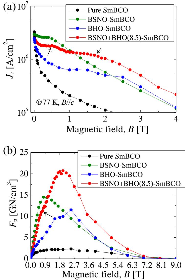
Fig. 6 Magnetic field dependence of (a)  $J_c$  and (b)  $F_p$  for pure, BSNO 32vol.%-doped, BHO 8.5vol.%-doped, BSNO 32vol.%+BHO 8.5vol.% co-doped SmBCO films at 77 K under magnetic fields applied parallel to the  $c$ -axis of SmBCO. In (a), the co-doped film shows a double  $J_c$  plateau, and end fields of the double plateau are pointed out by arrows in (a). A black arrow in (b) shows a shoulder at 0.7 T.
