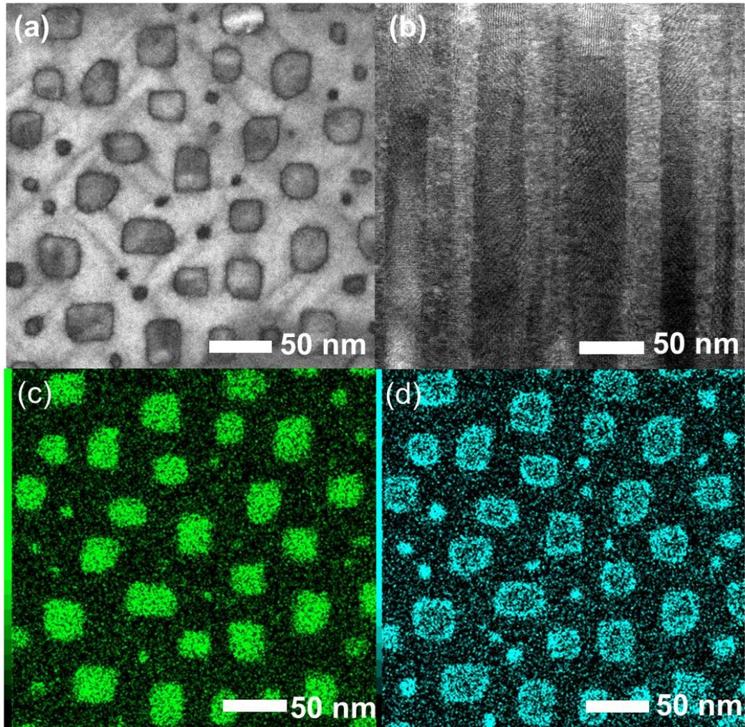
Fig. 4 (a) Plane view and (b) cross-sectional TEM images of BSNO 32vol.% and BHO 8.5vol.% co-doped SmBCO film. EDX elemental mappings of (c)Nb and (d) Hf for the plane view image.
