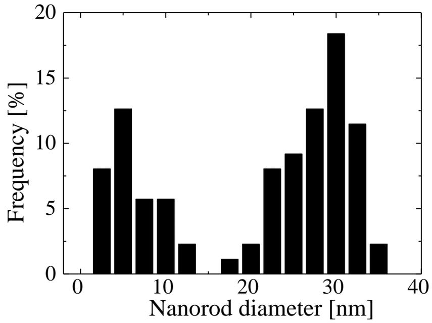
Fig. 5 Histogram of nanorod diameters for the SmBCO film co-doped with BSNO 32vol.% and BHO 8.5vol.%.
