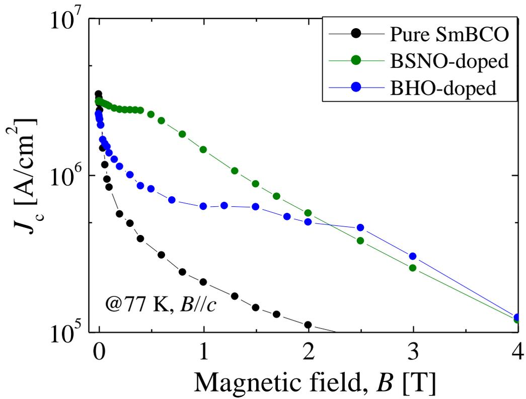
Fig. 3 Magnetic field dependence of  $J_c$  for pure, BHO 8.5vol.-%-doped and BSNO 32vol.-%-doped SmBCO films at 77 K under magnetic fields applied parallel to the  $c$ -axis of SmBCO.
