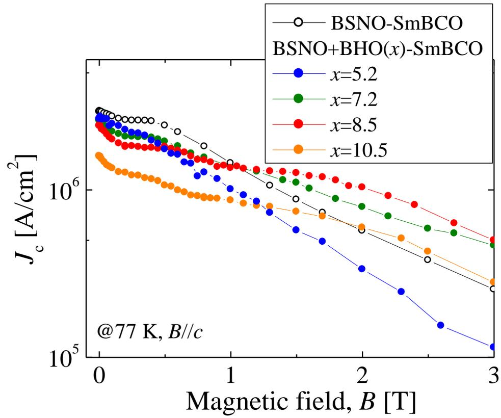
Fig. 8 Magnetic field dependence of  $J_c$  for BSNO 32vol.%+ BHO 5.2-10.5vol.% co-doped SmBCO films at 77 K under the fields applied parallel to  $c$ -axis of SmBCO.
