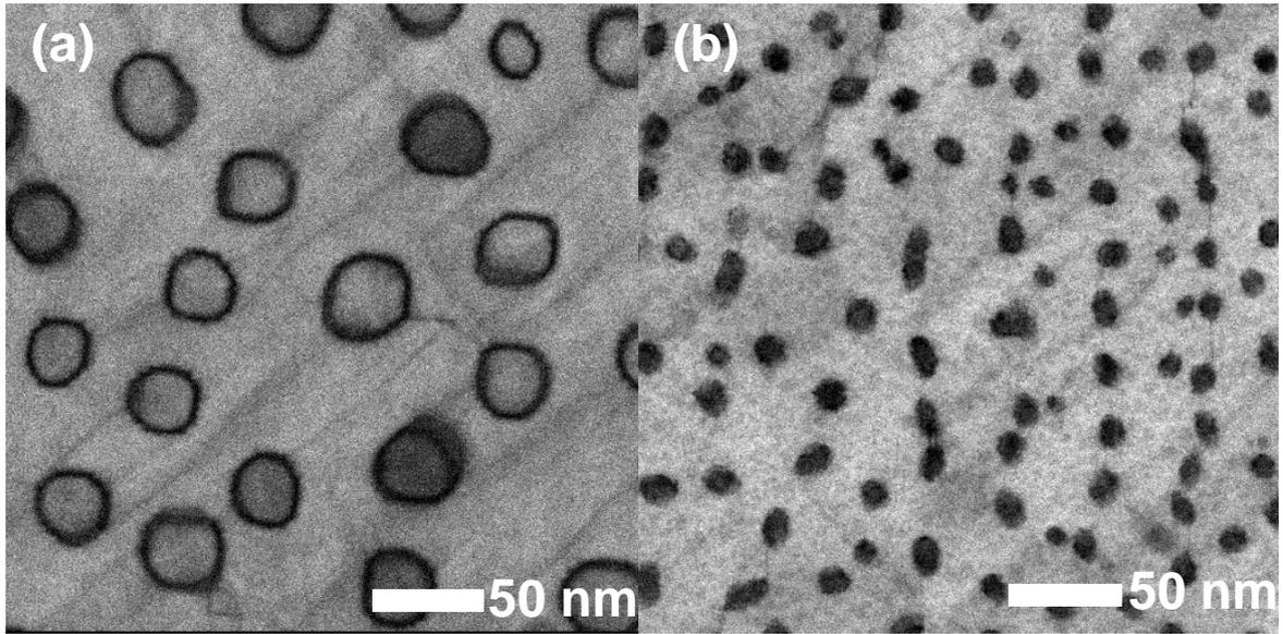
Fig. 2 Planer view of TEM images for (a) BSNO 32vol.%-doped SmBCO film, (b) BHO 8.5vol.%-doped SmBCO film.
