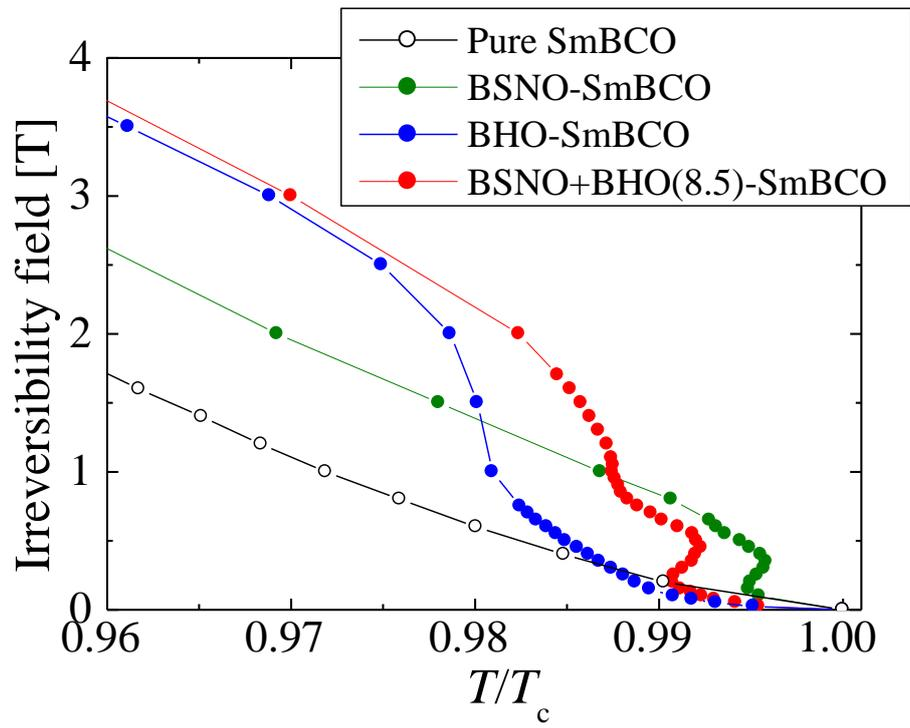
Fig. 7 Temperature dependence of irreversibility fields. Horizontal axis is normalized by each  $T_c$  at 0 T.
