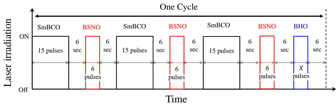
Fig. 1 Targets alternating cycle and irradiation pulse number for SmBCO, BSNO and BHO targets.
