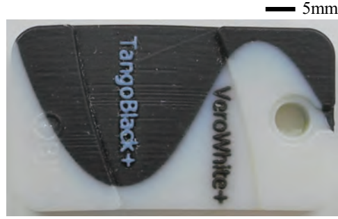
Figure 3: Example of an object fabricated from black and white materials by multi-material photopolymer additive manufacturing device.
