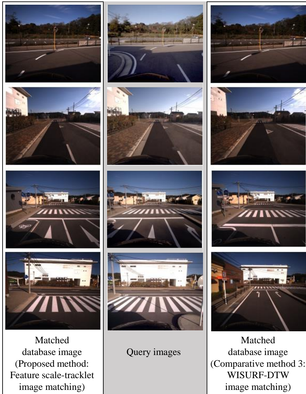
Figure 3.11: Example image matching results from the driving-school dataset. The top two rows show image matching in the same lane as the database lane, whereas the lower two show matching where the query lane is different from the database lane.
