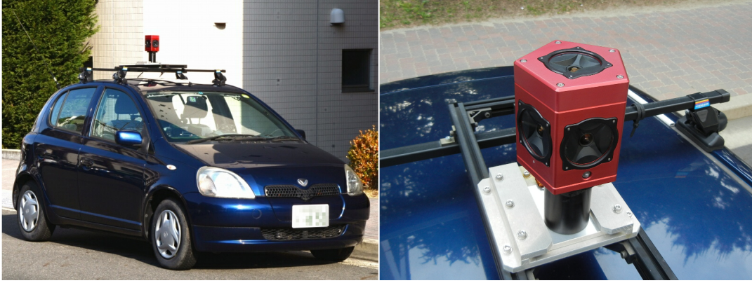
Figure 3.4: Point Grey Ladybug camera [96] mounted on the test vehicle.
