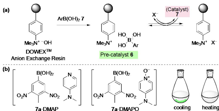
**Figure 1.** Novel boronic acid–base complexes as reusable homogeneous catalysts for amide condensation
