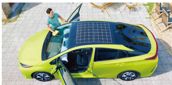
Fig.1.1: Plug-in hybrid vehicle with roof-top photovoltaics (source: TOYOTA Motor Corp.)
