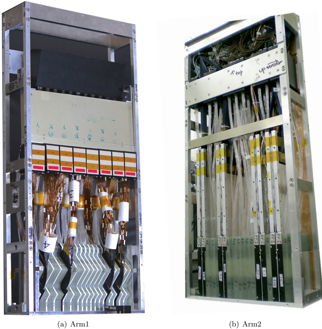
FIGURE 3.3: LHCf detectors Arm1 and Arm2. Calorimeter components including scintillators, tungsten plates and PMTs, position sensors and their front-end electronics are packed in a 92 \text{ mm}^w \times 620 \text{ mm}^h \times 280 \text{ mm}^l aluminum box.
