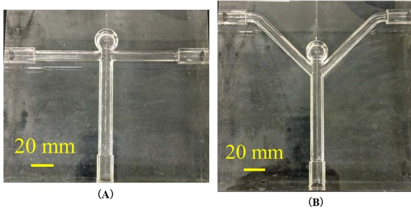
Fig. 3 Basilar artery aneurysm models for experiments. (A) Type A, (B) Type B.
