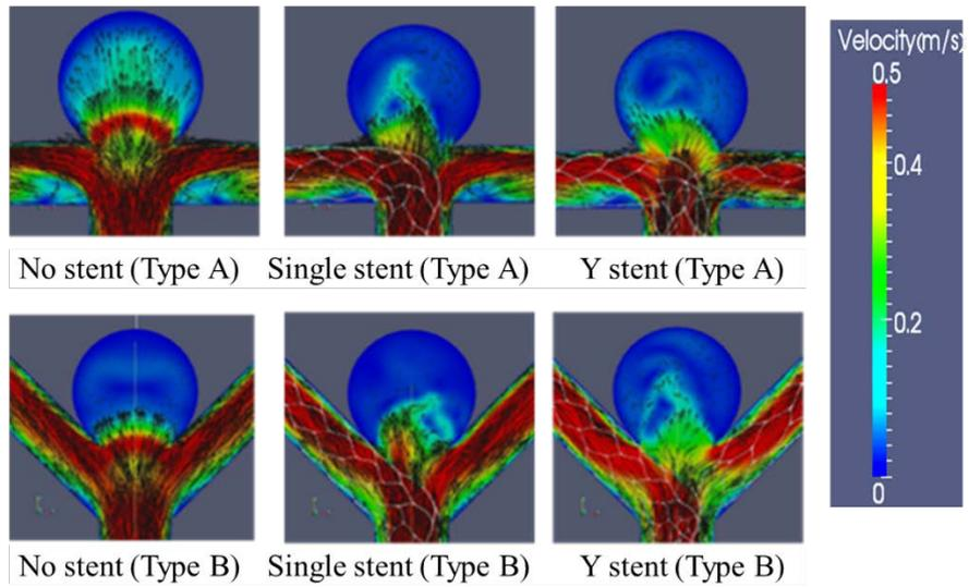
Fig. 8 Velocity vector and contour map at  $t = 0.3s$ .
