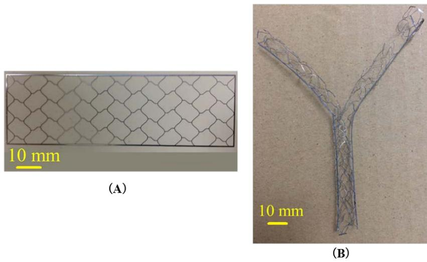
Fig. 4 Stent sheet and model. (A) Stent sheet of Enterprise VRD, (B) the Y stent model.
