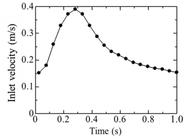
Fig. 2 Waveform of the inlet velocity for the CFD analysis.
