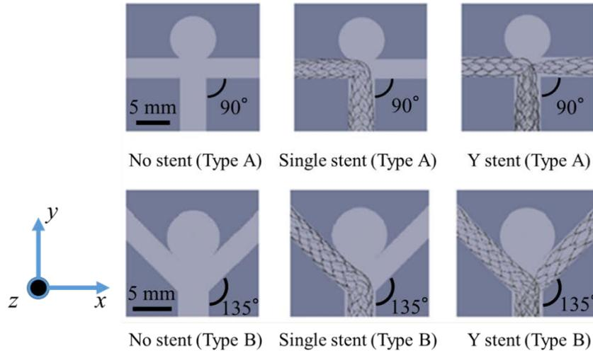
Fig. 1 Basilar artery aneurysm models and stent models for CFD simulations. The angle between basilar artery and posterior cerebral arteries is 90 and 135 degrees in Types A and B, respectively.
