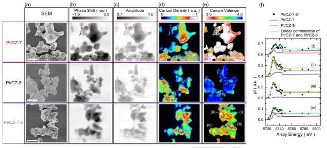
**Figure 2.** (a-e) Images of the Pt/CZ-7, Pt/CZ-8, and Pt/CZ-7.6 particles. The scale bar is 1 µm. (a) FE-SEM images. (b and c) Phase and amplitude images at 5.732 keV (d) Ce density maps. (e) Ce valence maps. The pixel size of the images in (b-e) is 13 nm. (f) One-pixel XANES spectra at particular positions (i)-(iv) marked in (e) of Pt/CZ-7.6. Red, blue, and green lines present the fitted spectra of Pt/CZ-7, Pt/CZ-8, and their linear combination, respectively.
