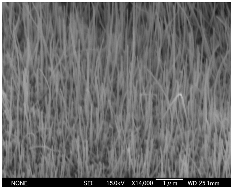
Fig. 5.10 \text{Fe}_2\text{O}_3 nanowire array after 20 seconds Ti sputtering
