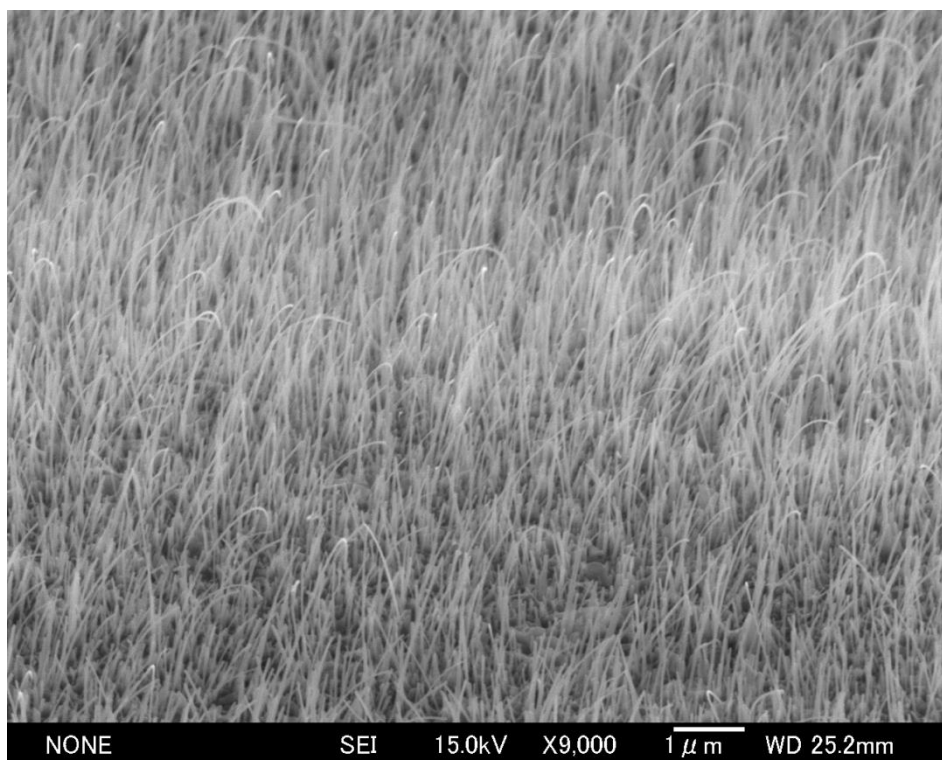
Fig. 5.2 Fe 2 O 3 nanowire array after 5 seconds Pt sputtering
