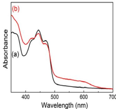
**Figure 1:** Absorption spectra of LOV-C254S in the presence of dithiothreitol (DTT) (a) before and (b) after illumination for 6 min. The sample concentration was 40  $\mu$ M.
