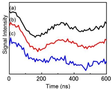
**Figure 4:** PELDOR signals of (a) LOV-C254S and (b) PZ-C254S without DNA and (c) with DNA. The signals were divided by the background signal as a linear function. The sample concentrations: (a) 220  $\mu\text{M}$ , (b) 260  $\mu\text{M}$  and (c) 150  $\mu\text{M}$ . Experimental conditions were the same as for Figure 3.
