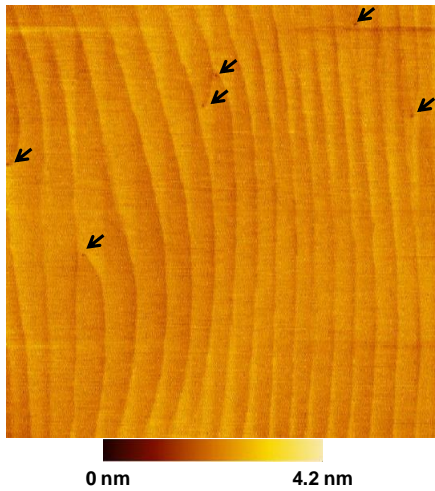
Figure 16 Surface AFM image of GaN layer when in-situ etching process was used. Area size was 3 \times 3 \mu\text{m}^2 . Black arrows indicate threading dislocation pits. Density of threading dislocations of GaN surface was estimated to be 6.7 \times 10^7/\text{cm}^2 .
