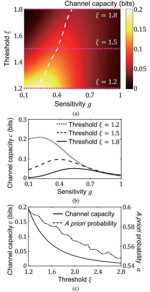
Fig. 2: (a) Channel capacity. Local maxima of the capacity in the dimension of the quantizer threshold  $\xi$  are shown by the white dashed line. (b) Channel capacities for the specific thresholds  $\xi = 1.2, 1.5$  and  $1.8$ . (c) Channel capacity and *a priori* probability on the ridge line in (a). The parameter settings are  $s_0 = \{0, 1\}$ ,  $\sigma_v^2 = 1$ , and  $\sigma_h^2 = 0.09$ .
