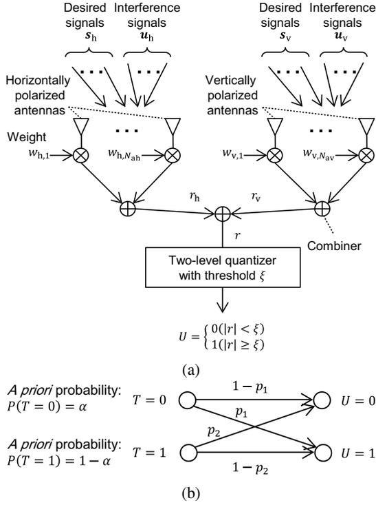
Fig. 1: (a) Schematic depiction of the interference-aided signal detection in the polarization diversity. (b) Binary asymmetric channel. Channel transition probabilities are expressed as  $P(U = 1|T = 0) = p_1$  and  $P(U = 0|T = 1) = p_2$ .
