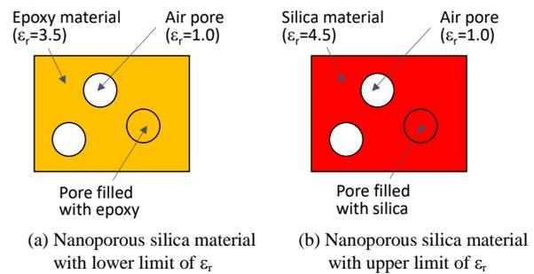
**Figure 9.** Assumptions of lower and upper limits of permittivity for nanoporous silica material whose nanopores are partially filled with epoxy resin.
