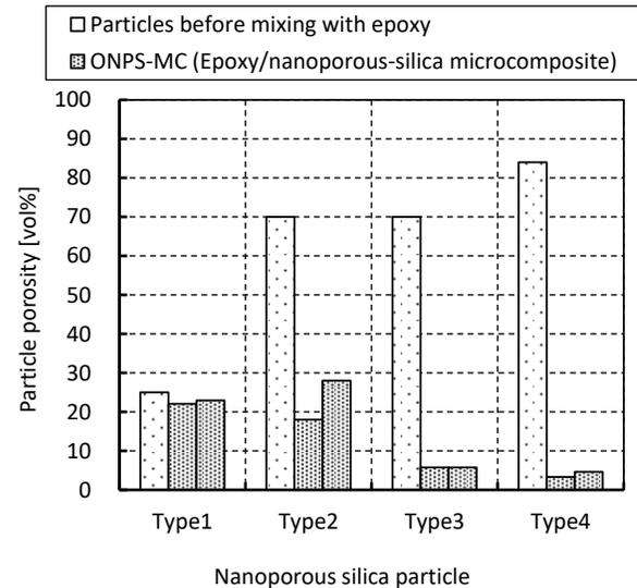
**Figure 6.** Porosity of open nanoporous silica fillers (Types 1-4) before mixing with epoxy and those filled with ONPS-MCs.
