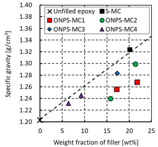
**Figure 2.** Specific gravity of unfilled epoxy, S-MC, and ONPS-MCs for different silica filler contents by weight.
