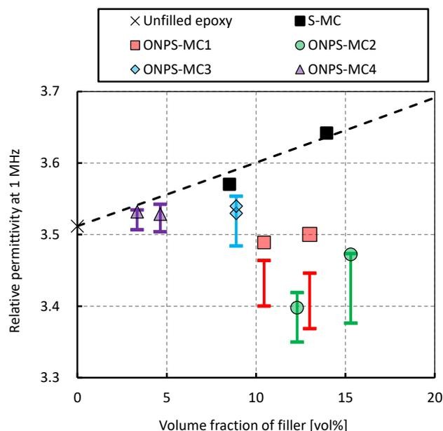
**Figure 10.**  $\epsilon_r$  at 1 MHz with different silica filler content by volume for unfilled epoxy, S-MC, and ONPS-MCs. The two horizontal marks indicated on the vertical lines are calculated values obtained from the model with the estimated lower and upper limits of permittivity for mesoporous silica material with the nanopores partially filled with epoxy.
