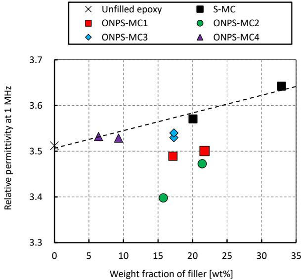
**Figure 5.** Relative permittivity at 1 MHz of unfilled epoxy, S-MC, and ONPS-MCs with different silica filler contents by weight.
