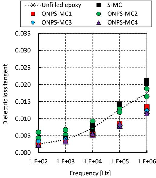
**Figure 4.** Frequency dependence of dielectric loss tangent of unfilled epoxy, S-MC, and ONPS-MCs.
