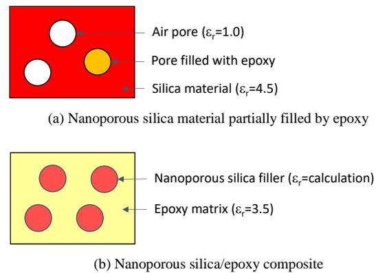
**Figure 8.** Schematics of epoxy composite with nanoporous silica filler whose nanopores are partially filled with epoxy resin.
