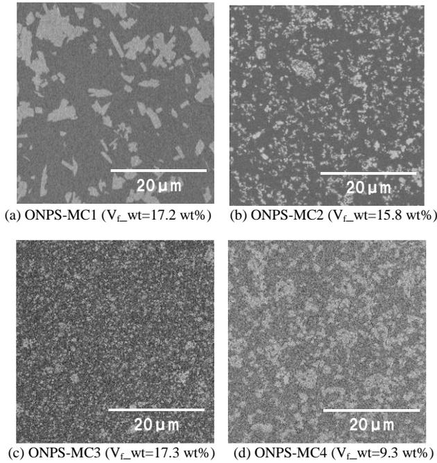
**Figure 1.** SEM images of epoxy/open nanoporous silica microcomposites (ONPS-MC1-4).  $V_{f\_wt}$  is the weight fraction of the filler.
