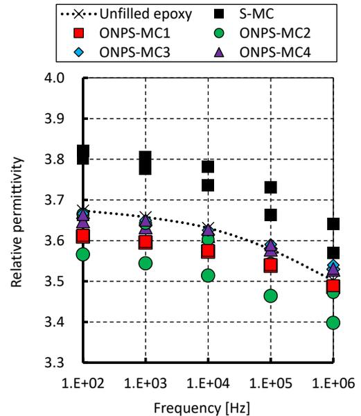
**Figure 3.** Frequency dependence of relative permittivity  $\epsilon_r$  of unfilled epoxy, S-MC, and ONPS-MCs.
