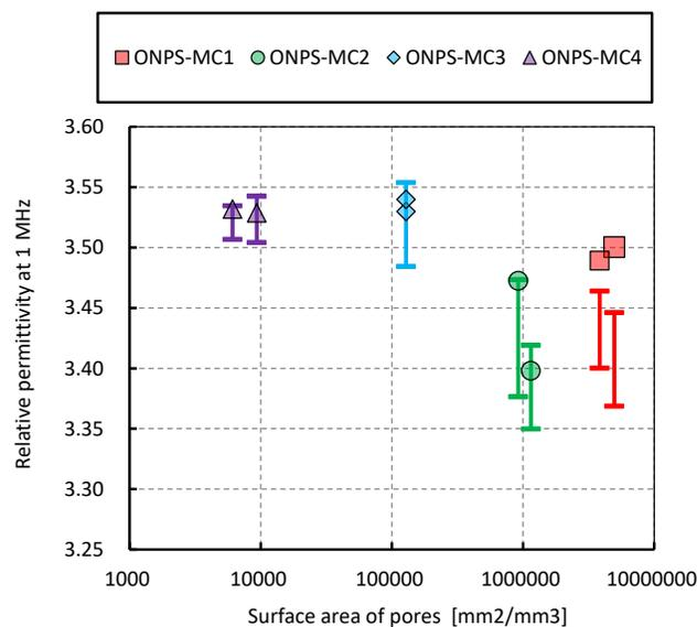
**Figure 11.**  $\epsilon_r$  at 1 MHz with different surface areas of pore. The two horizontal marks indicated on the vertical lines are calculated values obtained from the model with the estimated lower and upper limits of permittivity for mesoporous silica material with the nanopores partially filled with epoxy.
