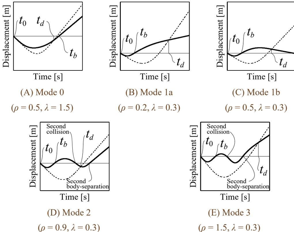
Figure 6. Schematic representations of one-dimensional collision vibration modes. (**bold**: displacement of the body mass; thin-dashed: displacement of the damper mass)
