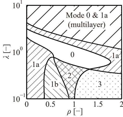
Figure 7. MEID one-dimensional collision vibration modes. ( $M = 1$  kg,  $K = 1$  kN/m,  $v_0 = 1$  m/s)
