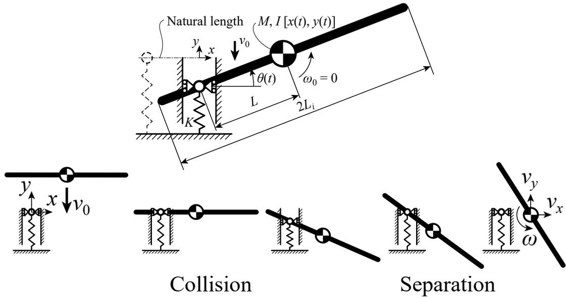
Figure 12. Object-wall-collision of a mass.
