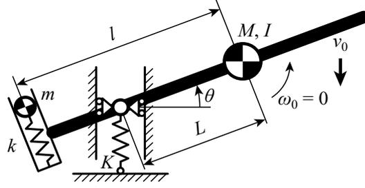
Figure 13. Two-dimensional collision model of MEID.
