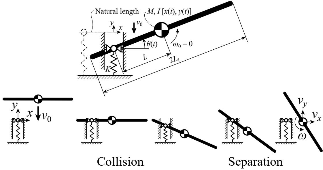
Figure 12. Object-wall-collision of a mass.
