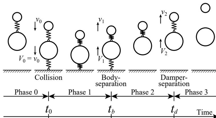
Figure 4. Schematic representation of the mechanical transitions of one-dimensional motion MEID collisions.
