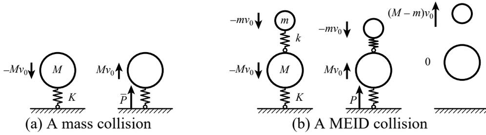
Figure 8. Momentum transfer of a mass and MEID collision.
