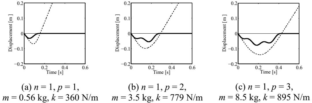
Figure 5. Typical responses of an optimal MEID in one-dimensional motion.
