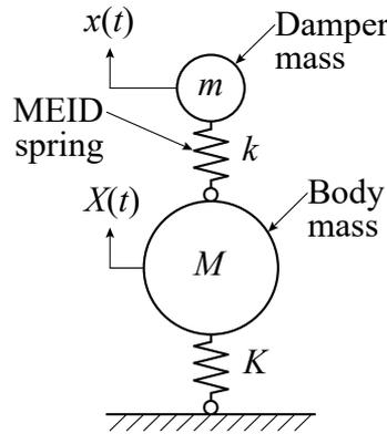
Figure 3. MEID model of a one-dimensional collision.
