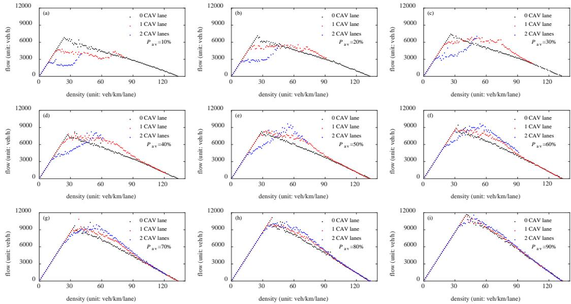
Fig. 2. Flow-density diagrams under different CAV dedicated lanes policies,
