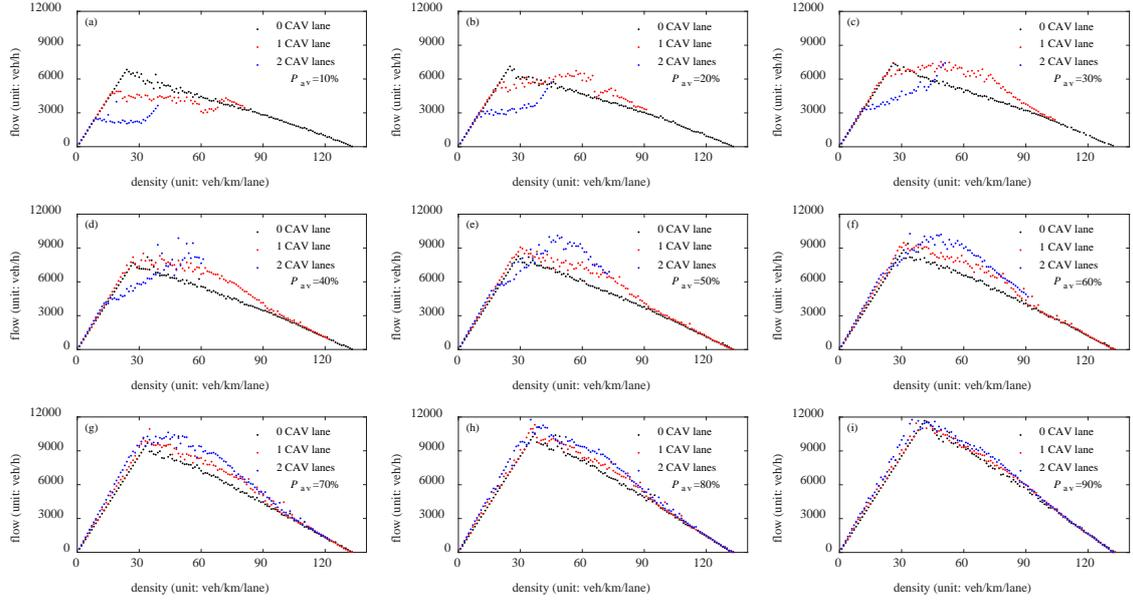
Fig. 5. Flow-density diagrams under different CAV dedicated lanes policies, with a higher maximum speed of CAV on the dedicated lanes. Each subplot corresponds to a CAV penetration rate  $P_{av}$ , which increase from 10% to 90%,
