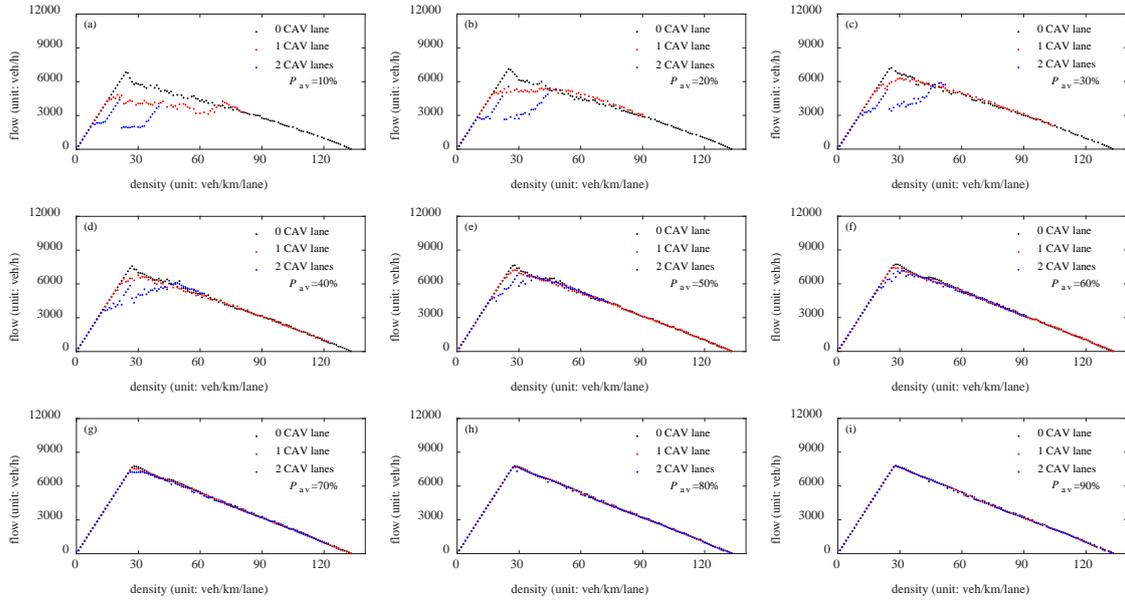
Fig. 4. Flow-density diagrams under different CAV dedicated lanes policies,
