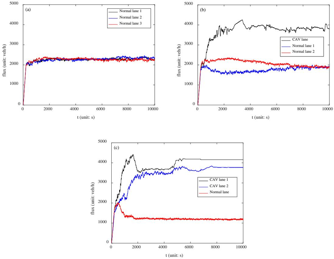
Fig.1. Flow-time diagrams under different CAV dedicated lanes policies  $P_{av}=60\%$ , vehicle density is 60 veh/km/lane,  $T_{ACC} = 0.5$  s. (a) 0 CAV dedicated lane, (b) 1 CAV dedicated lane (c) 2 CAV dedicated lanes.
