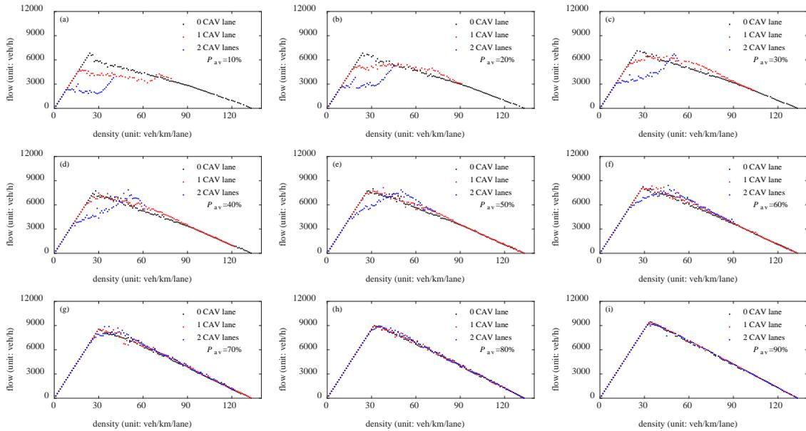
Fig. 3. Flow-density diagrams under different CAV dedicated lanes policies,
