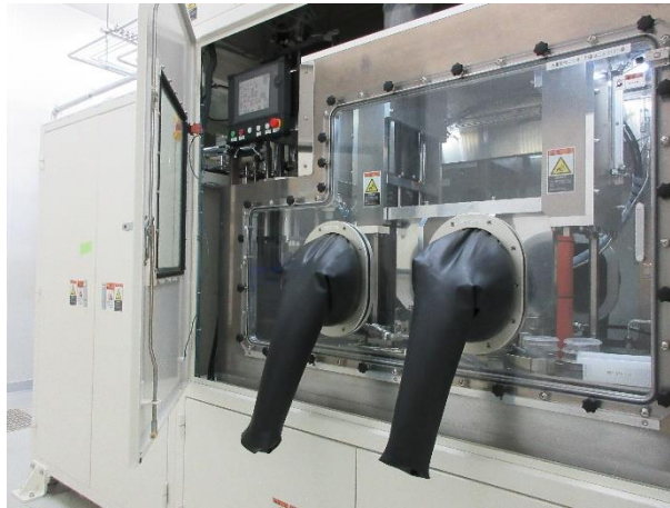
Fig. 2.1 Photograph of TAIYO NIPPON SANSO MOVPE SR-2000 system.
