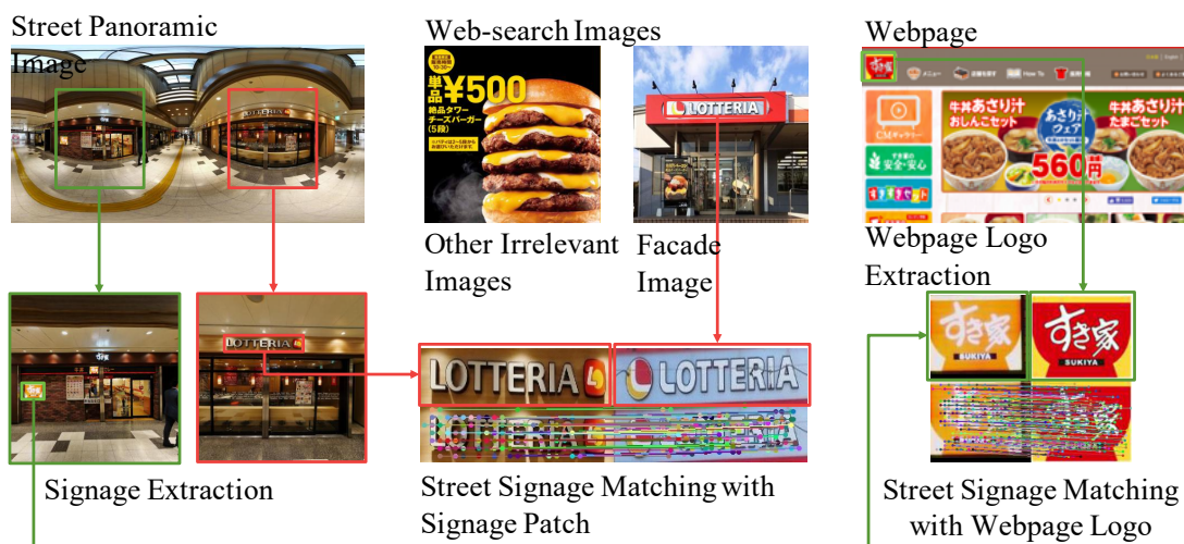
Figure 6.7: Example of the signage identification process. Two image patches (‘LOTTERIA’ and ‘SUKIYA’) are cropped out from street images as query images. The ‘LOTTERIA’ patch is matched with a similar looking signage patch, which is extracted and cropped from thousands of other Web search images. The ‘SUKIYA’ image is matched with the official ‘SUKIYA’ logo, which proposed logo extraction method had effectively extracted from its Website.
