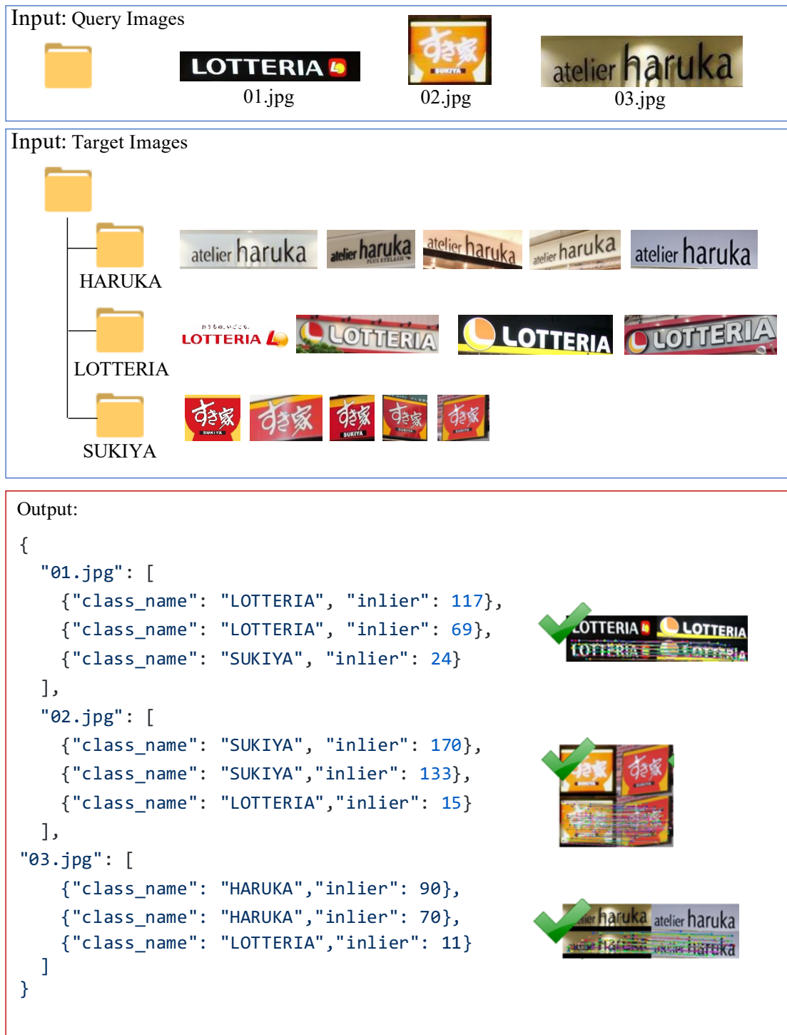
Figure 6.11: Example of inputs and outputs of the Hybrid Image Matching algorithm.
