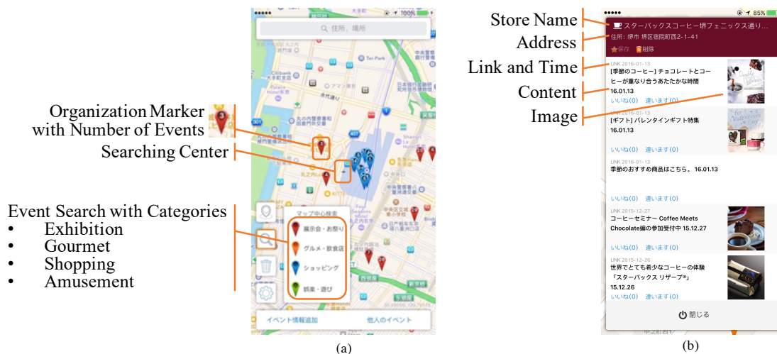
Figure 4.3: Main interfaces of the Event.Locky application. (a) markers with the number of event records of stores, museums, etc. on an electronic map; search coordinate is set at the center of the map (the cross marker), which by default is set to the current location obtained from a built-in GPS sensor. It can also be indicated by dragging on the map. (b) Detailed event records are listed after touching a marker sorted by event time.
