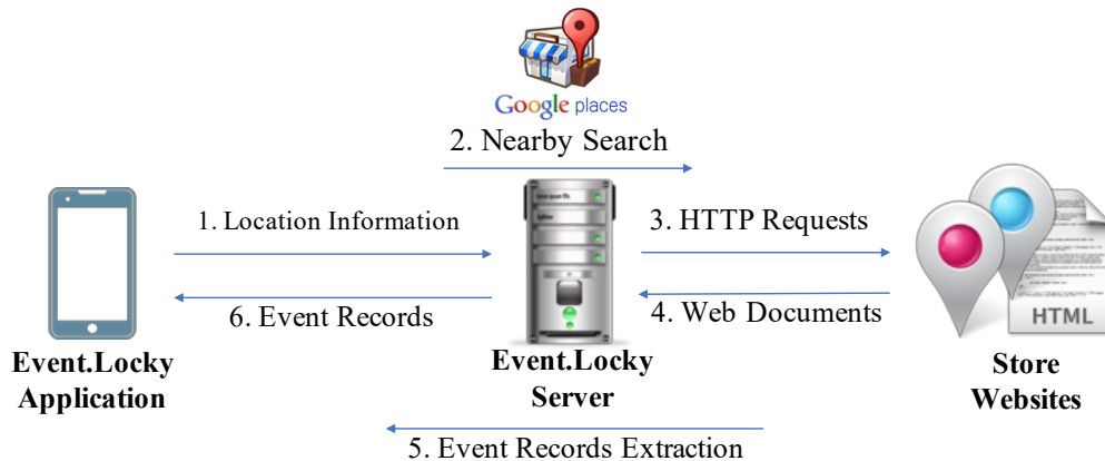
Figure 4.2: Processing flow of the Event.Locky application.
