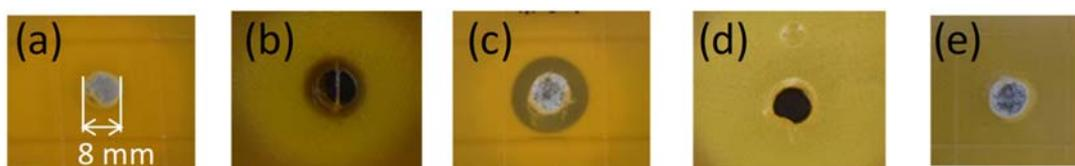
**Fig. 1** Bioassay of polymer colloids prepared using the following monomers and initiators: (a) MMA and V-50; (b) Styrene and V-50; (c) Styrene and VA-044; (d) Styrene and AIBN; (e) Styrene and KPS. The white particles seen at the centers of the images are the polymeric particle sediments.
