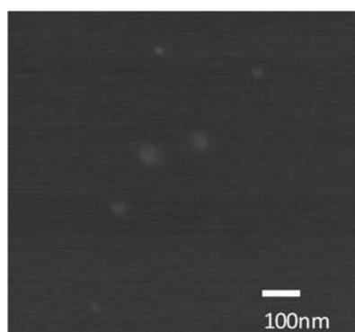
**Fig. 3** SEM image of the supernatant polymers, obtained through soap-free emulsion polymerization of styrene with 2.03 mM VA-044, adsorbed electrostatically on the mica surface.
