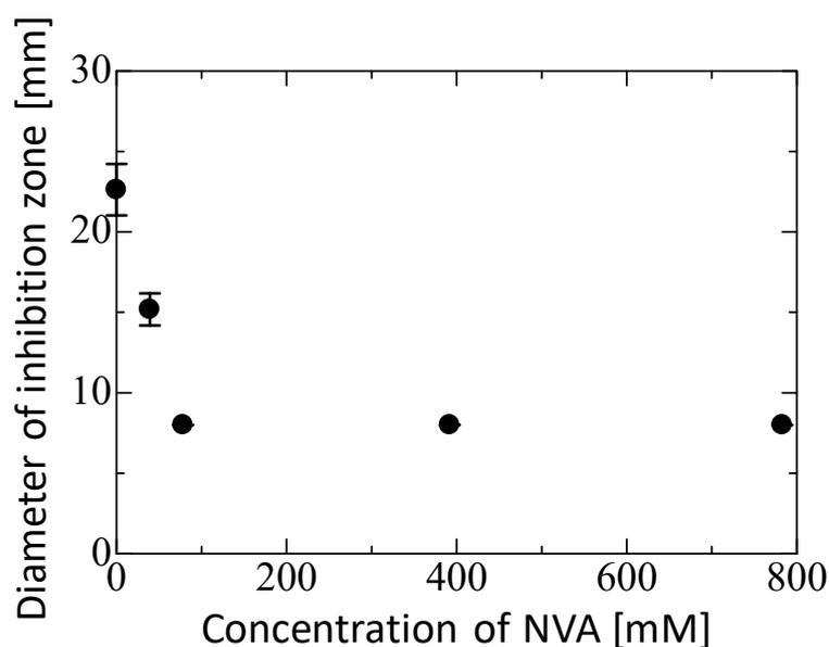
**Fig. 7** Influence of the NVA concentration used in the polymerization of styrene with V-50 on the inhibition zone examined by a bioassay test using the supernatant. The 8 mm diameter dots indicate the diameter of the inhibition zone for the present sample.
