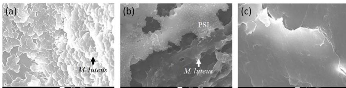
**Fig. 6** SEM images of the polystyrene plates modified with: (a) no polymer; (b) polymer materials obtained through centrifugal separation; (c) polymers remaining in the supernatant after the bioassay. The scale bars correspond to 1 μm.
