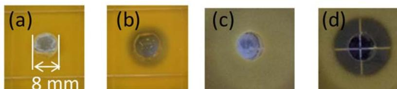
**Fig. 2** Results of the bioassays of particles or supernatant prepared using the following monomers and initiators: (a) particles with size of 180 nm synthesized using styrene and V-50; (b) supernatant obtained using styrene and V-50; (c) particles with size of 108 nm synthesized using styrene and VA-044; (d) supernatant obtained using styrene and VA-044.
