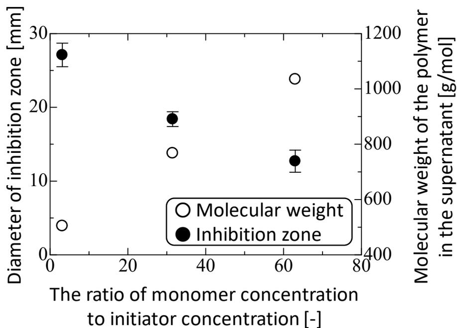
**Fig. 4** Influence of the ratio of monomer concentration to initiator concentration on the molecular weight of the synthesized polymer dissolved in the supernatant, inhibition zone examined via a bioassay test.
