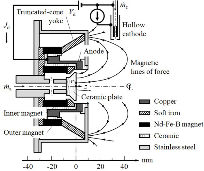
**Fig. 1. Schematic of diverging magnetic field electrostatic thruster.**
