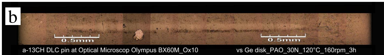
Figure 3.2-3 Wear scar on a-C:H coated pins after friction and wear tests for 2h and 3h under 20N and 30N load.
