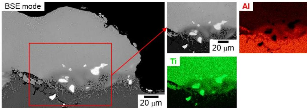
**Fig. 6** EDS elemental mapping of the porous layer formed with Al-Ti powder blend
