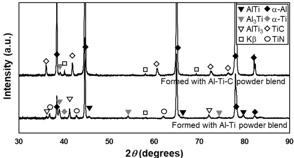
**Fig. 5** X-ray diffraction patterns of the porous layers formed with different powder blends
