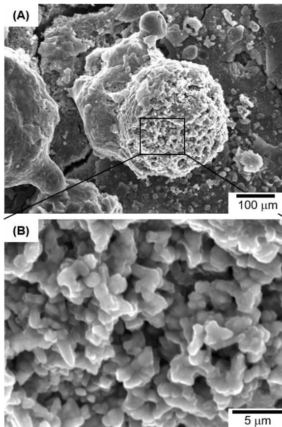
**Fig. 8** Etched particle-shaped protrusion in the porous layer formed with Al-Ti-C powder blend. (A) low- and (B) high-magnification view.
