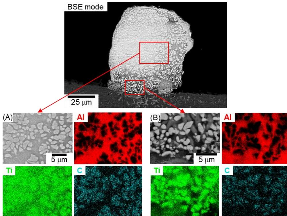
**Fig. 7** EDS elemental mapping of the porous layer formed with Al-Ti-C powder blend. (A) middle region and (B) near substrate region.
