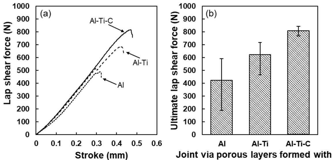
**Fig. 10.** (a) Lap shear force-stroke curves and (b) ultimate lap shear force of Al/PA6 joints fabricated via different porous layers. Error bar shows the maximum and minimum values obtained from three samples.
