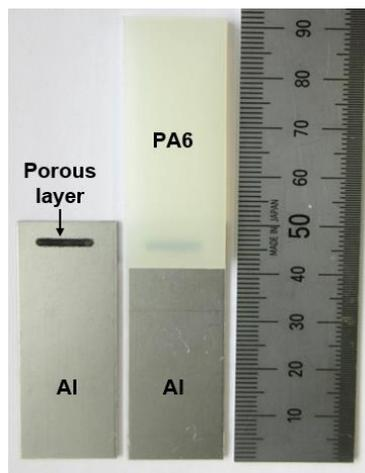
**Fig. 3** Photographs of an Al substrate with a porous layer (left) and an Al/PA6 joint (right).
