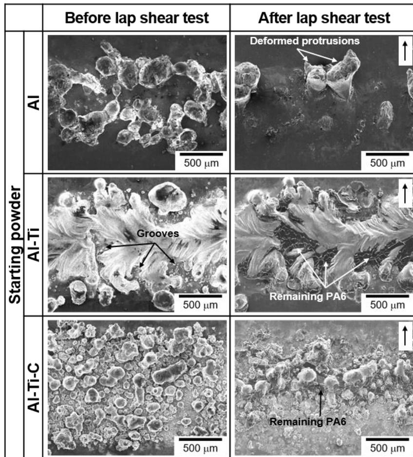
**Fig. 11** SEM images of the porous layer before and after lap shear test (Black arrow in white box shows the direction of the applied shear force)
