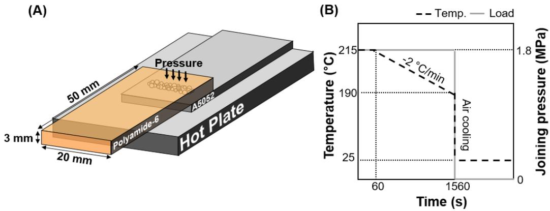
**Fig. 2** (A) Schematic illustration of the Al/PA6 joint fabrication process. (B) History of the temperature of the sample stage and joining pressure.
