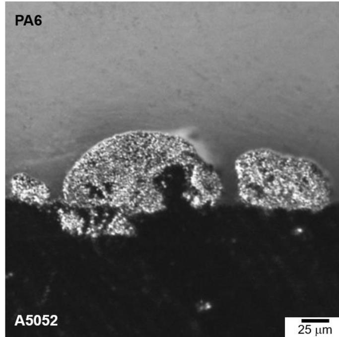
**Fig. 9** Optical micrograph of the cross-section of an Al/PA6 joint
