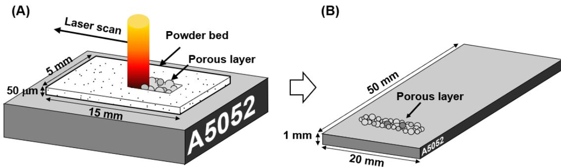
**Fig. 1** Schematic illustration of the porous layer formation process on the Al alloy (A5052) substrate. (A) laser irradiating process and (B) after ultrasonic cleaning
