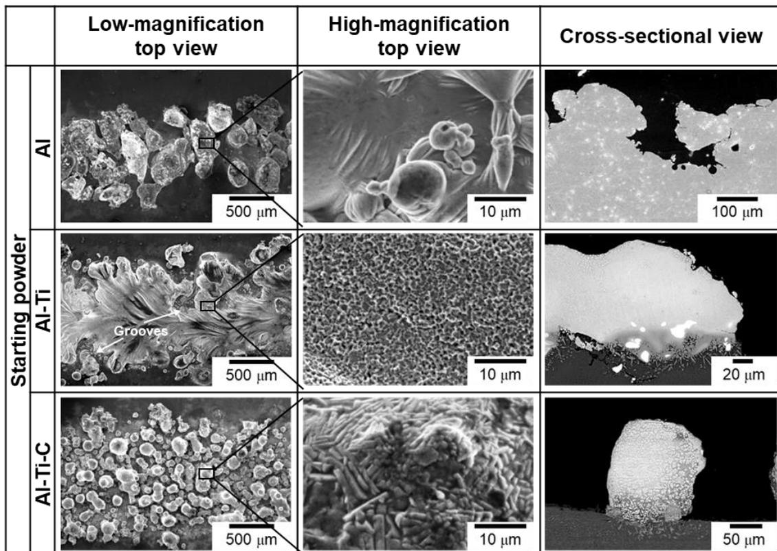
**Fig. 4** Low- and high-magnification top view, and cross-sectional view of the porous layers
