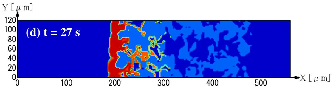
Fig. 6. Profiles of soot deposition region at different times obtained of bare DPF.
