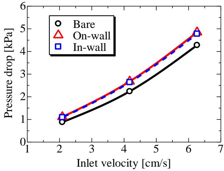
Fig. 2. Initial pressure drop of bare DPF, on-wall CDPF, and in-wall CDPF obtained by experiments.
