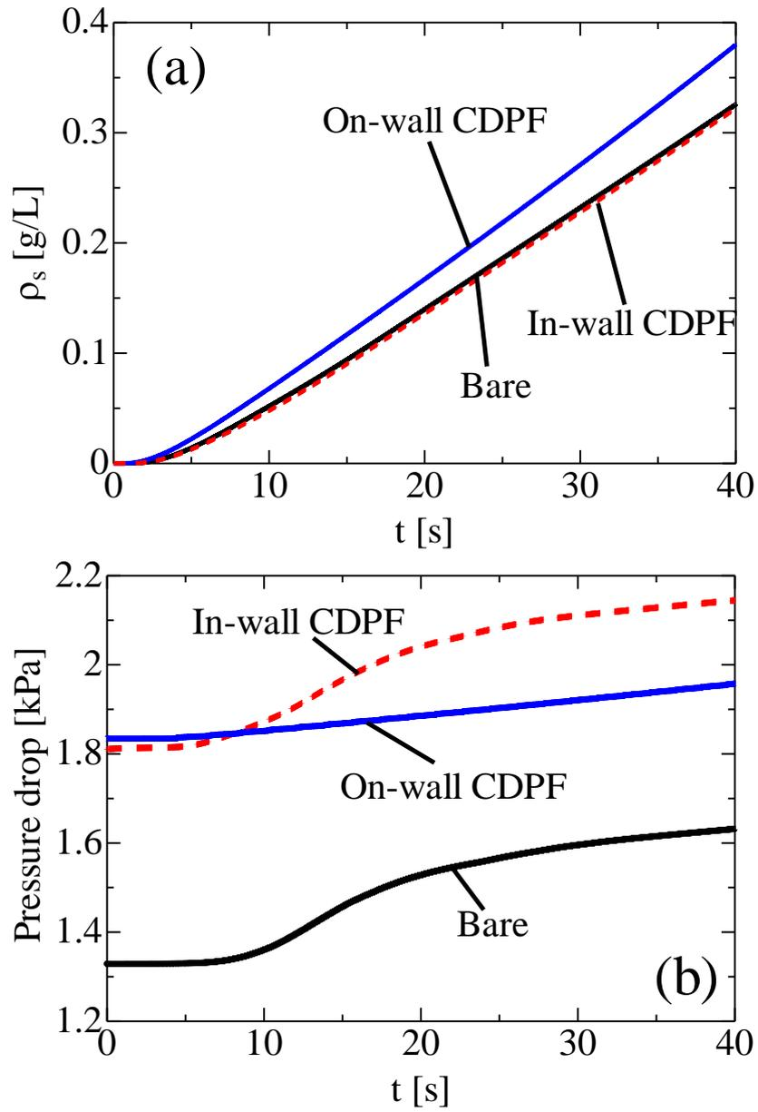
Fig. 9. Time-variations of (a) soot amount and (b) pressure drop
