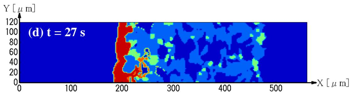
Fig. 7. Profiles of soot deposition region at different times obtained of in-wall CDPF.
