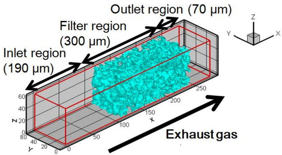
Fig. 1 Numerical domain with coordinate system.
