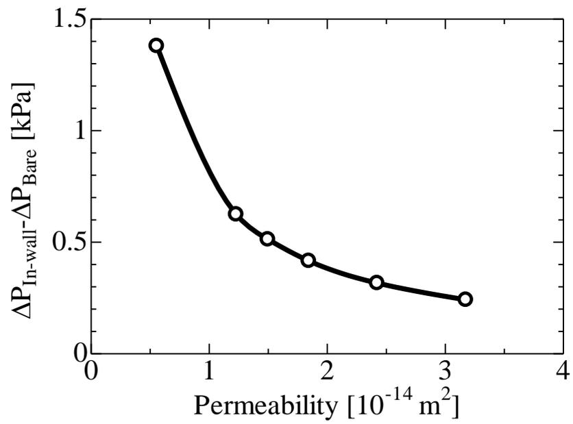
Fig. 3. Numerical results are shown to see difference between the initial pressure drops of bare DPF and in-wall CDPF when the permeability of the catalyst layer was changed.
