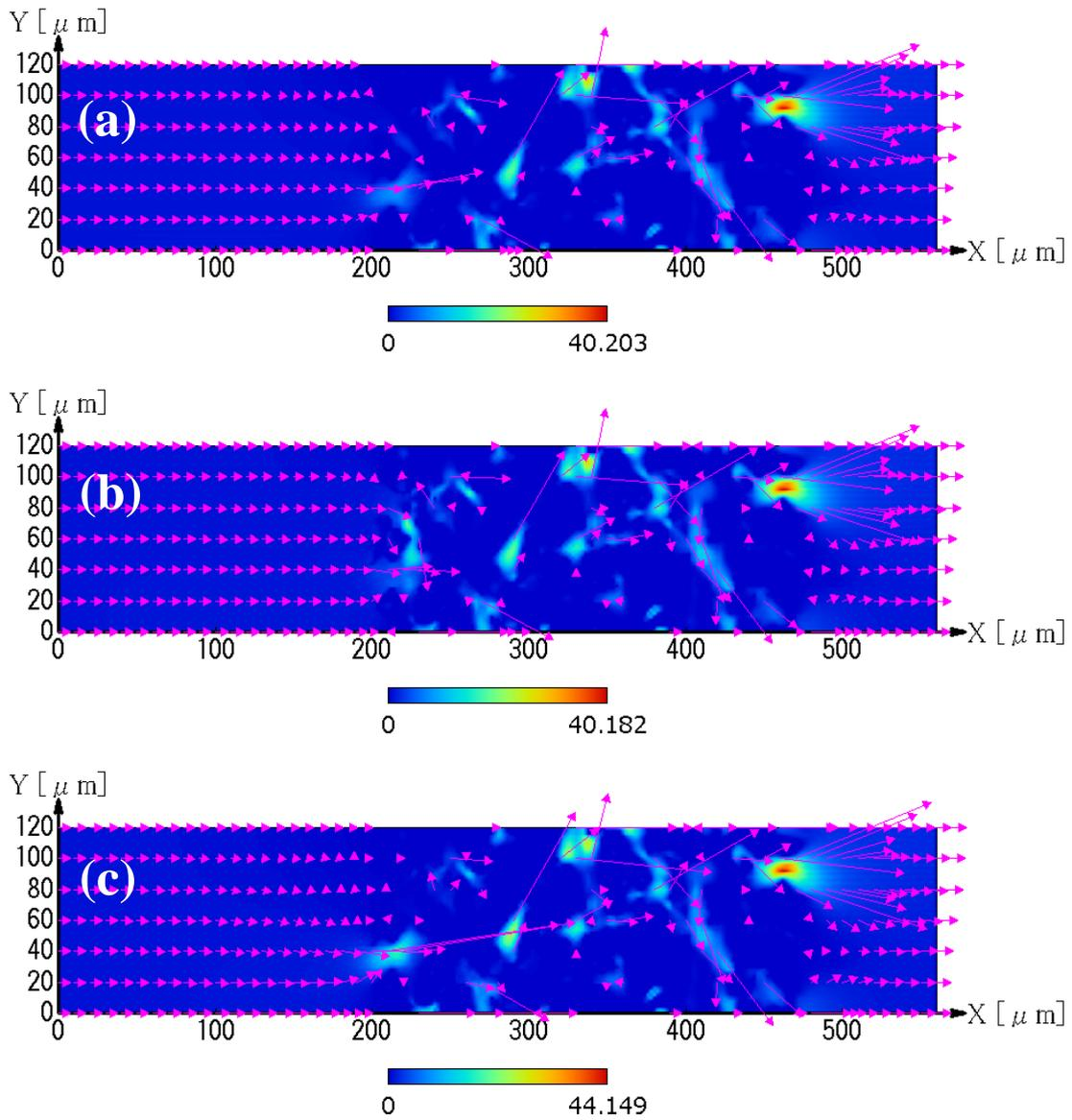
Fig. 4. Flow fields of (a) bare DPF, (b) on-wall CDPF, (c) in-wall CDPF.
