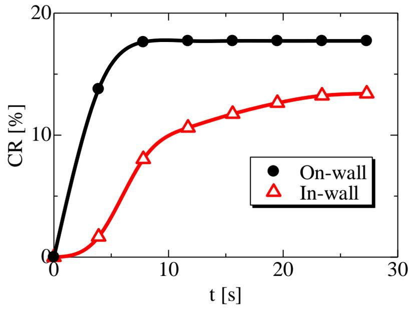
Fig. 10. Time-variation of the contact ratio of in-wall and on-wall CDPFs
