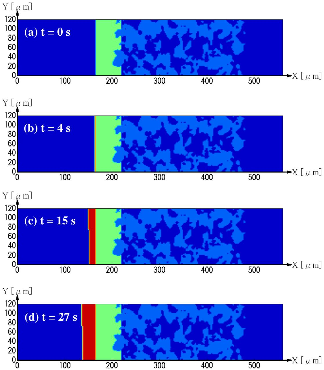
Fig. 8. Profiles of soot deposition region at different times obtained of on-wall CDPF.
