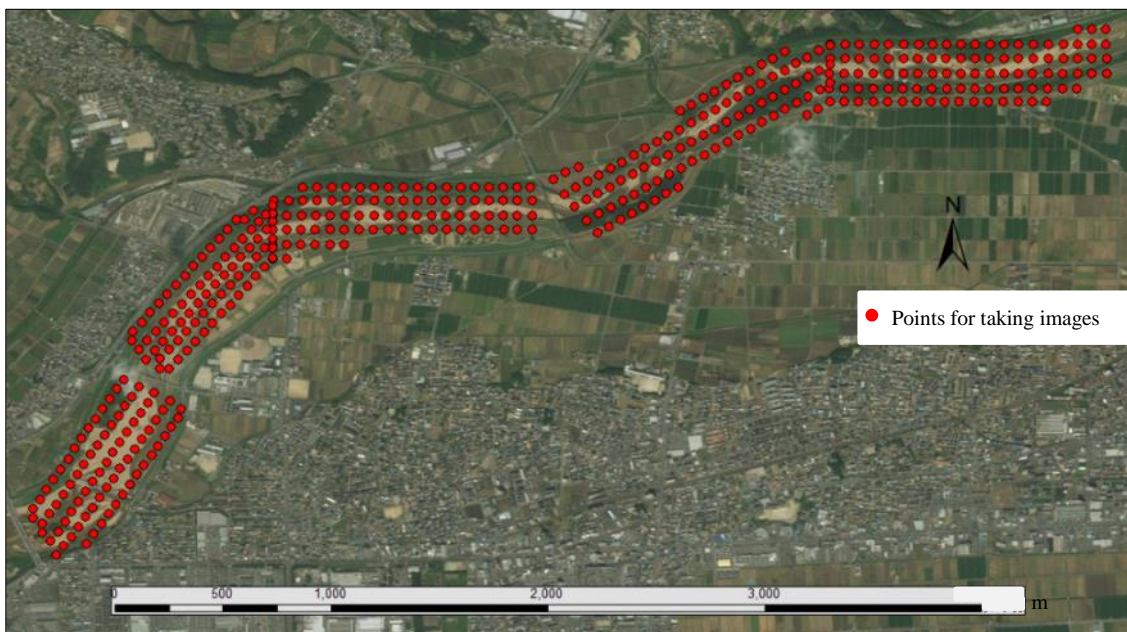
Figure 3.2 Points setting for taking UAV images
