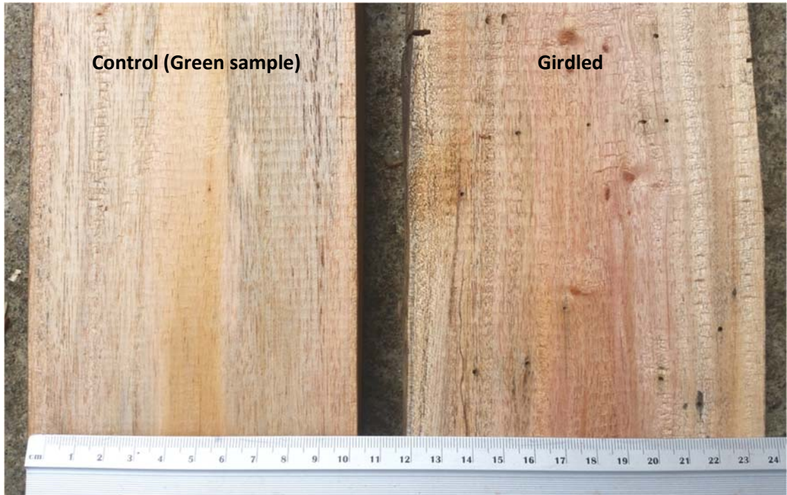
Figure 4-10. Wood color difference of control (green samples)(left) and girdled treatment (right). Color difference is \Delta E^*_{ab} = 18.72 (small diameter).
