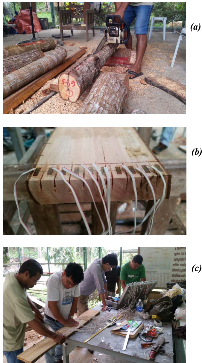
Figure 3-2.a. Collection of wood samples and measurement: Preparation of wood samples (a), Installation of strain gages (b) and measurement of radial release strain (c)
