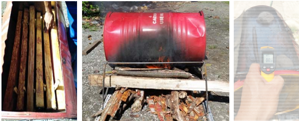
Figure 5-2.b. Water heated set up using the steel drum and firewood to fuel the water at heating temperature of 80°C accumulated in 48 hours.
