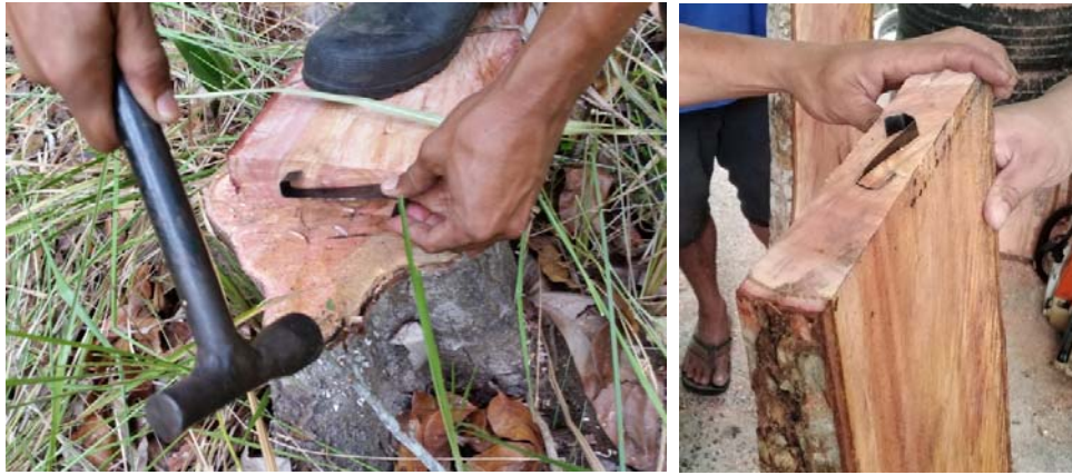
Figure 5-2.a. Application of lumber clip to arrest cracking (release strain) during sawing.
