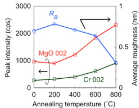
Fig. 2. MgO 002 and Cr 002 peak intensities and average surface roughness  $R_a$  of the buffer structure Cr (10 nm) / MgO (20 nm) / CrB (5 nm) / NiTa (25 nm) /  $\text{SiO}_2$  / Si sub. as a function of the annealing temperature.
