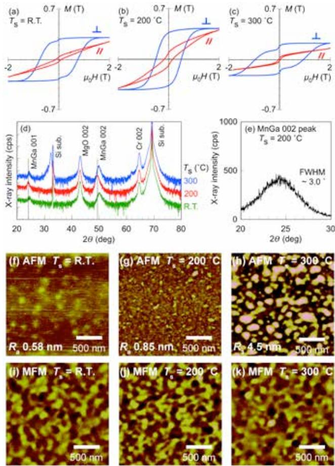
Fig. 3. (a) – (c)  $M$ - $H$  curves, (d) XRD patterns, (e) rocking curve of MnGa 002 peak, (f) – (h) AFM images, and (i) – (k) MFM images of MnGa films grown on the Cr buffer layer annealed at  $T_a^{\text{Cr}} = 600$  °C. The substrate temperature  $T_s$  during the growth of MnGa layer was varied at R.T., 200, and 300 °C. The dashed lines in Fig. (d) show the peak positions of the bulk MnGa.
