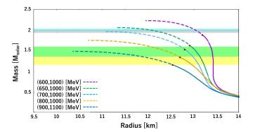
FIG. 11. Relation between the mass and radius of neutron stars for several combinations of two chiral invariant masses in group 4. The curves are for  $(m_0^{(1)}, m_0^{(2)}) = (600, 1000), (650, 1000), (700, 1000), (800, 1000), (900, 1100)$  MeV from top to bottom.
