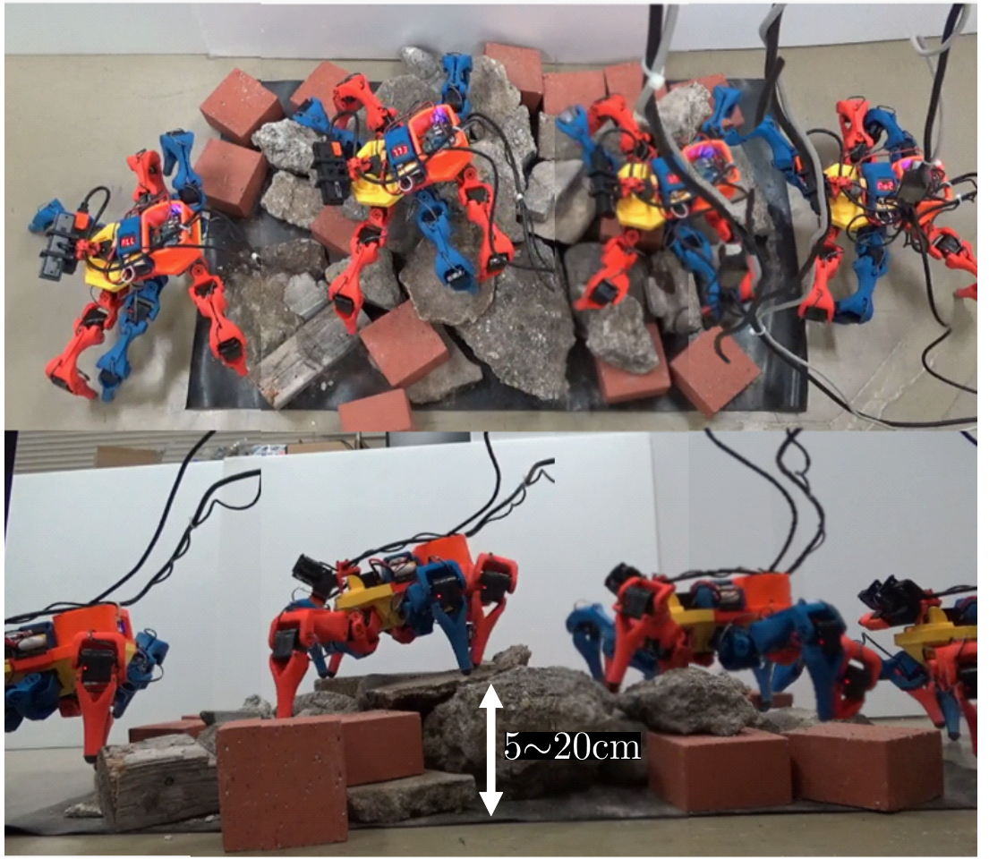
Fig. 6.4 Upper and side view of experiment with original FCP gait and Timekeeper control
