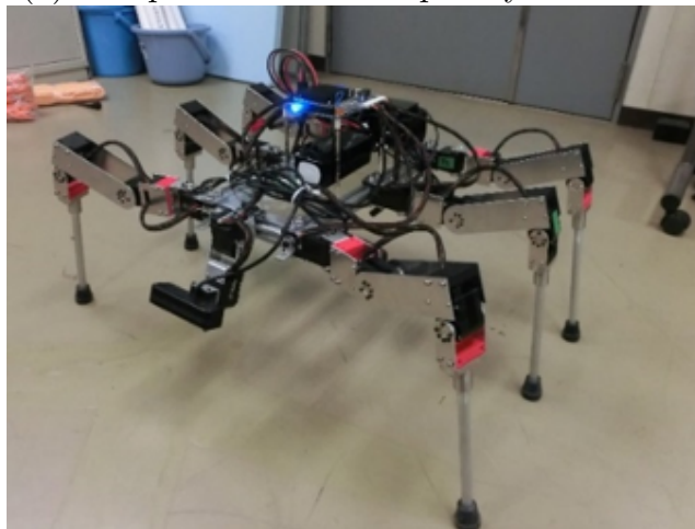
(b) Hexapod robot developed by Kishi and Kurita
