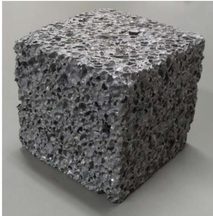
Fig.1-1 Image of typical porous Al [1-44].
