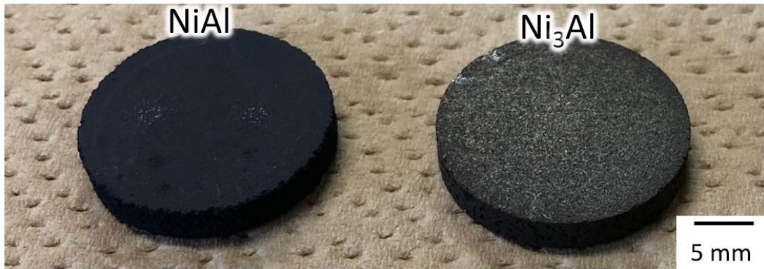
Fig. 5-2 Appearances of the representative sintered samples for permeability test.
