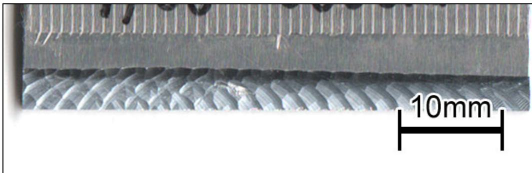
(12) Radial immersion of 60 deg ( \bar{\theta}_{im} = 60 deg) at spindle speed of 6000 min -1 evaluated as chatter (×) the workpiece has moved
