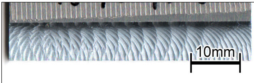
(3) Radial immersion of 60 deg ( \bar{\theta}_{im} = 60 deg) at spindle speed of 4800 min -1 evaluated as chatter (×)
