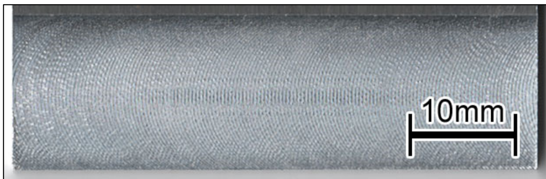
(3) Radial immersion of 150 deg ( \bar{\theta}_{im} = 150 deg) at spindle speed of 5200 min -1 evaluated as no chatter (○)
