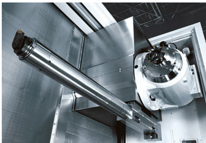
Fig. 1 - 2 Machine tool with special long boring bar[1-19]
