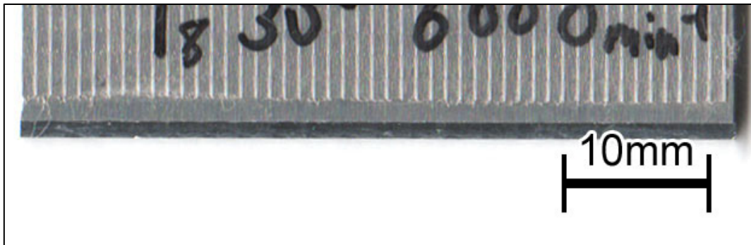
(11) Radial immersion of 30 deg ( \bar{\theta}_{im} = 30 deg) at spindle speed of 6000 min -1 evaluated as no chatter (○)
