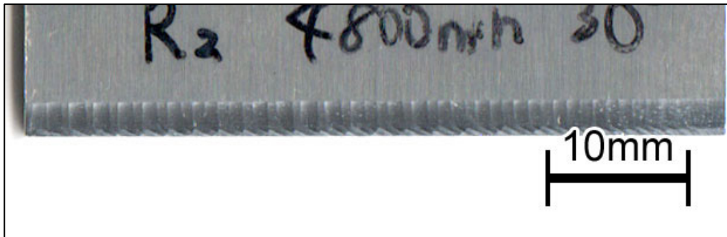
(1) Radial immersion of 30 deg ( \bar{\theta}_{im} = 33 deg) at spindle speed of 4800 min -1 evaluated as chatter (×)
