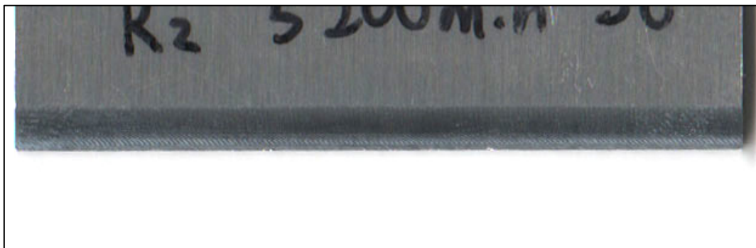
(2) Radial immersion of 30 deg ( \bar{\theta}_{im} = 33 deg) at spindle speed of 5200 min -1 evaluated as no chatter (○)
