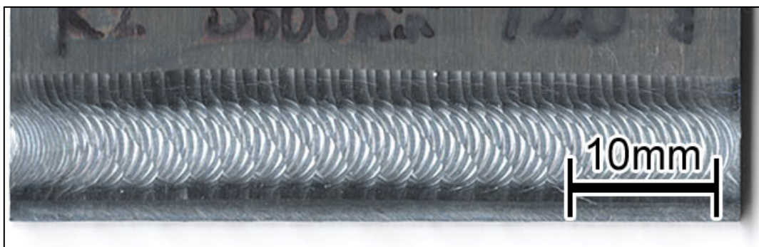
(6) Radial immersion of 120 deg ( \bar{\theta}_{im} = 142 deg) at spindle speed of 5600 min -1 evaluated as chatter (×)
