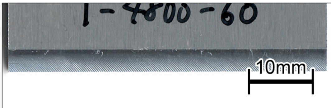
(2) Radial immersion of 60 deg ( \bar{\theta}_{im} = 60 deg) at spindle speed of 4800 min -1 evaluated as no chatter (○)
