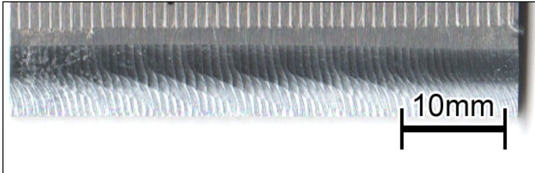
(4) Radial immersion of 90 deg ( \bar{\theta}_{im} = 100 deg) at spindle speed of 5200 min -1 evaluated as chatter (×)
