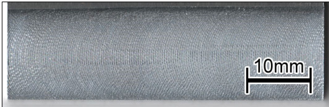
(1) Radial immersion of 150 deg ( \bar{\theta}_{im} = 150 deg) at spindle speed of 4800 min -1 evaluated as no chatter (○)
