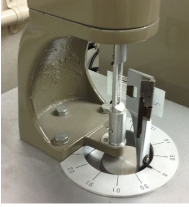
Figure 18: Measuring device for bending moment. Model No. KES-F2 (Kato-Tec Co., Ltd).
